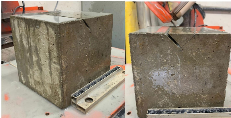
Figure 2. Cutting the triangular grooves.
