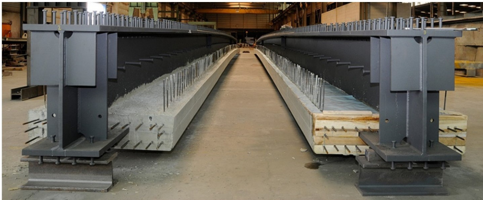
Figure 3. Pre-cambered composite beams, Preflex [10].
