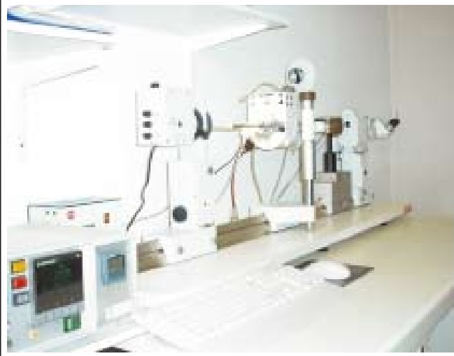
Figure 12. The heating microscope. On an optical bench the following major components are mounted (from left to right): Light source, vertical tubular furnace (max. 1650°C), video camera. At the lower left the programming and control unit is shown. The picture analysing system is not shown.
