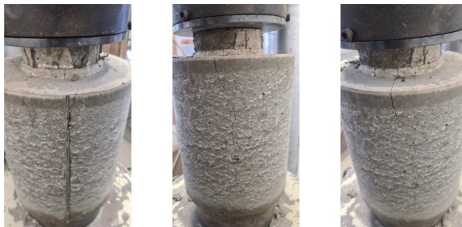
Figure 25. Longitudinal crack in a specimen with t = 4.6\text{cm} / H = 10\text{cm}
