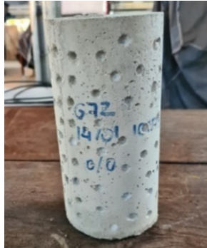
Figure 6. Mechanical chipping surface treatment (holes with drill)
