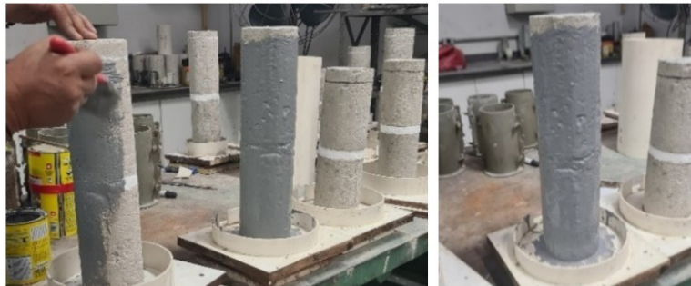
Figure 7. Epoxy adhesive surface treatment
