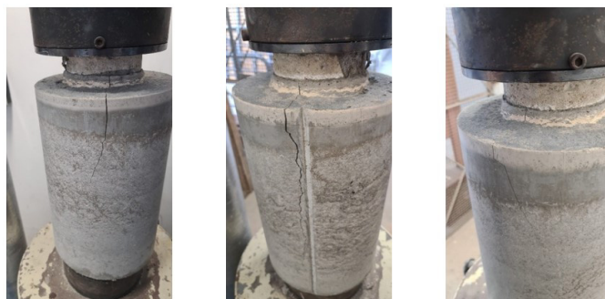
Figure 26. Longitudinal crack in a specimen with t = 4.6\text{cm} / H = 14\text{cm}
