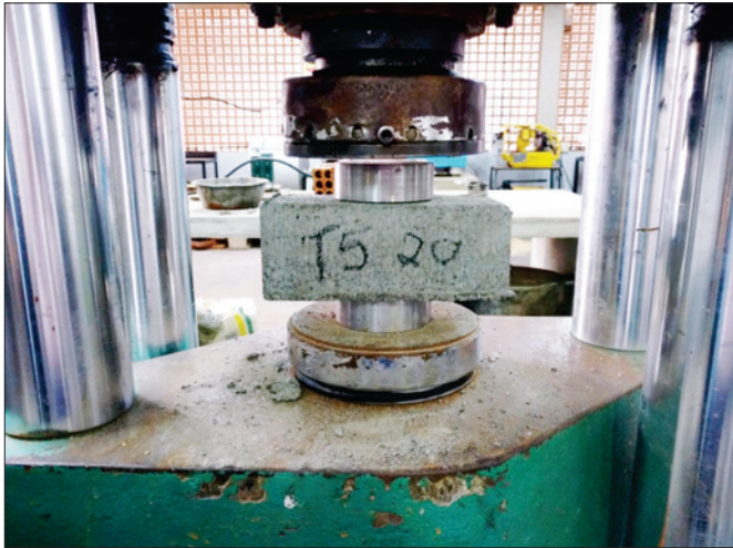
Figure 6 Paver in the press between the discs
