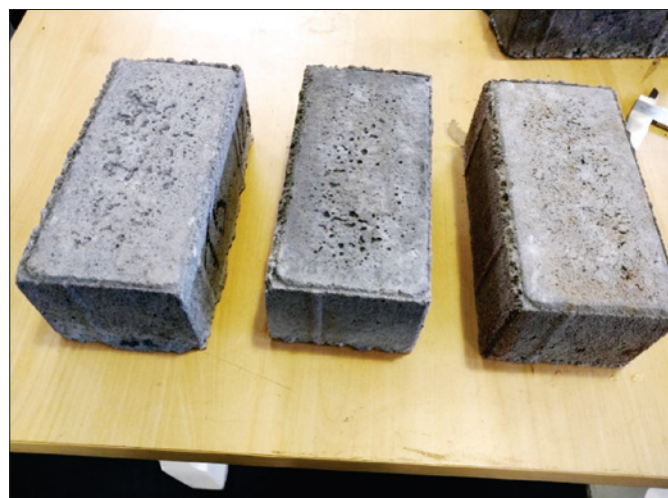
Figure 13 Pavers made from waste
