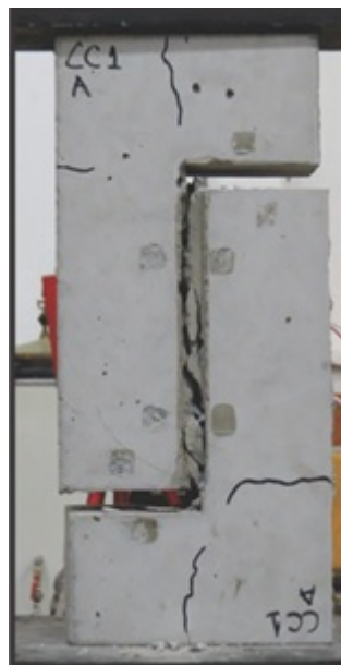
Figure 6. Rupture of specimen CC-A.
