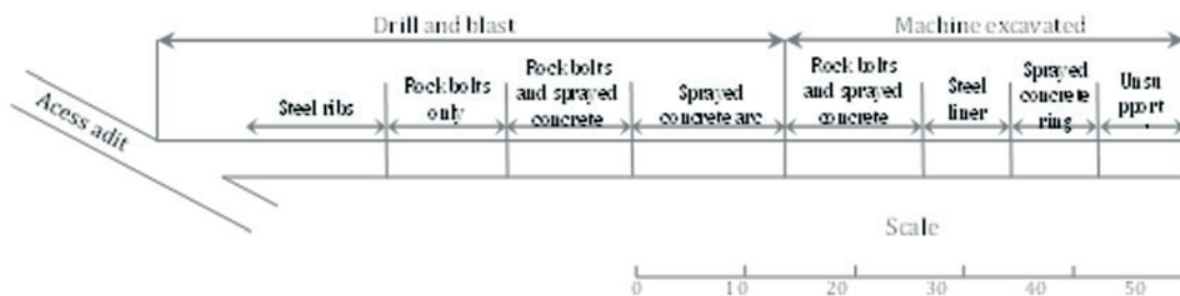
Figure 14 – Sections through the experimental Kielder tunnel. Freeman (13)
