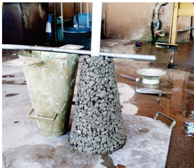
Figure 4 Slump test with zero slump
