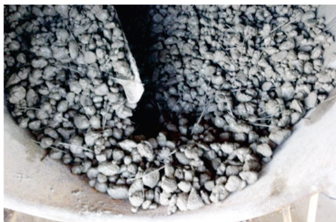
Figure 2 Appearance of the pervious concrete in mixture D1
