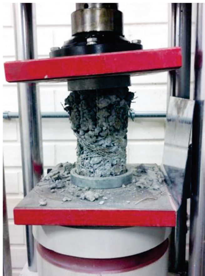
Figure 6 Rupture under axial compression of pervious concrete with fibers
