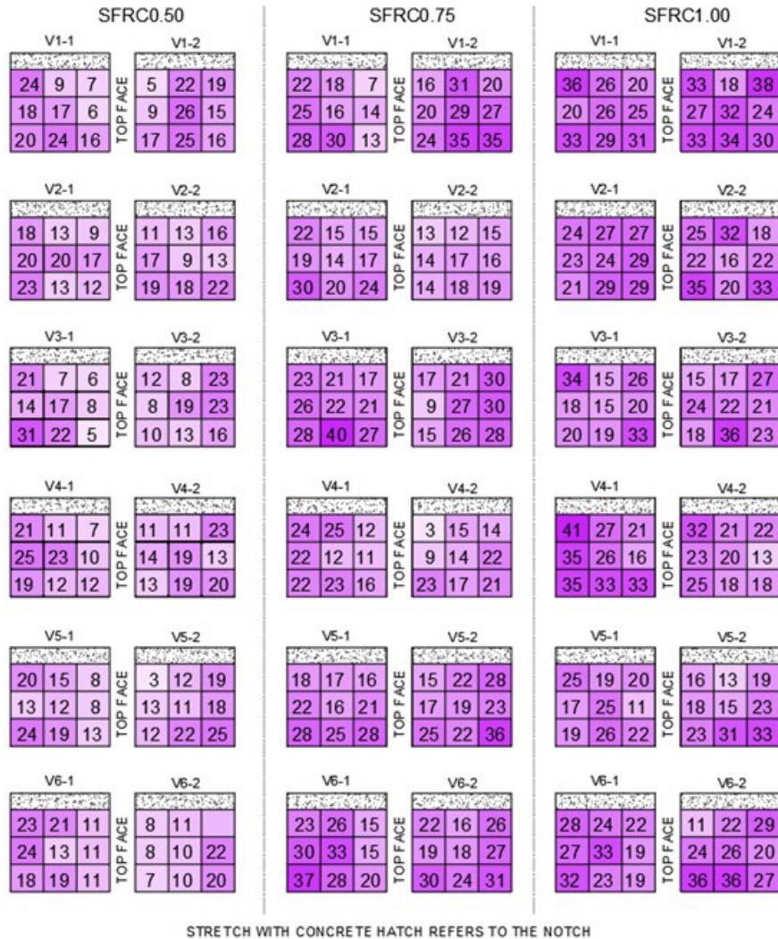
Figure 12. Fiber distribution in the prismatic specimens.
