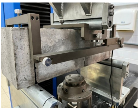
Figure 5. Flexural beam test.
