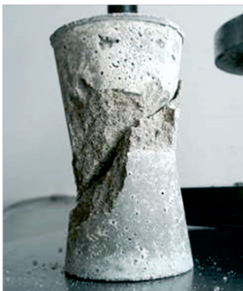
Figure 10 - Hourglass: shear plane mode of failure
