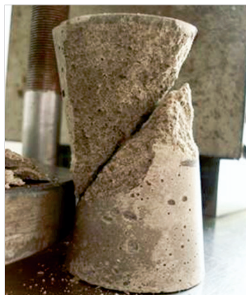
Figure 10 - Hourglass: shear plane mode of failure
