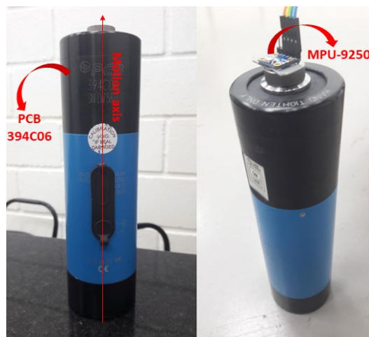
Figure 3. Testing setup (MPU-6050 attached to the calibrator).
