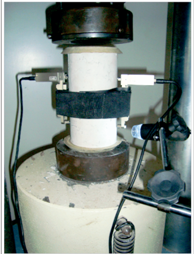
Figure 5 - Real setup of the experiment using a servo-hydraulic machine EMIC, Model PC 200 and an USB microscope (800x). The sample is also affixed with traditional strain gauges (mechanical extensometer)
