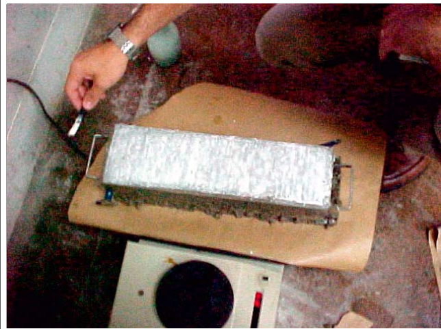
Figure 2 - Paraffin membrane applied over specimen surface
