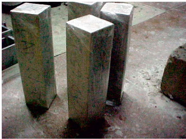
Figure 1 - Beam specimen sealed with PVC membrane
