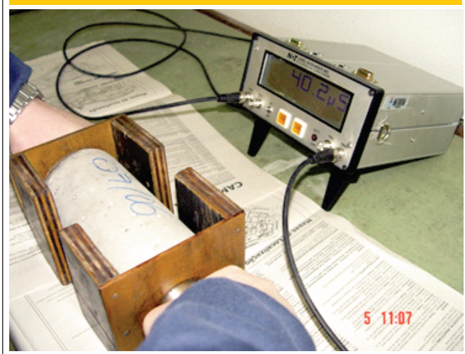
Figure 1 - Aspect of the performance of an UPV test
