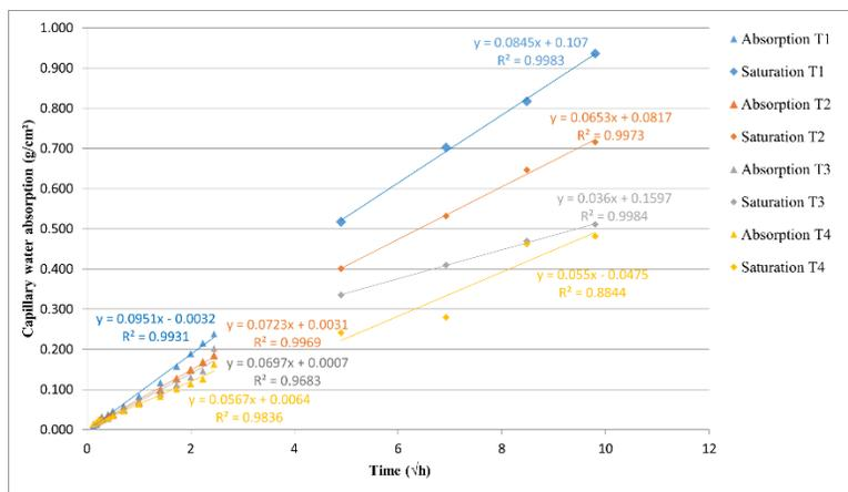
Figure 5. Capillary water absorption at 84 days for the concrete mixtures of this study.
