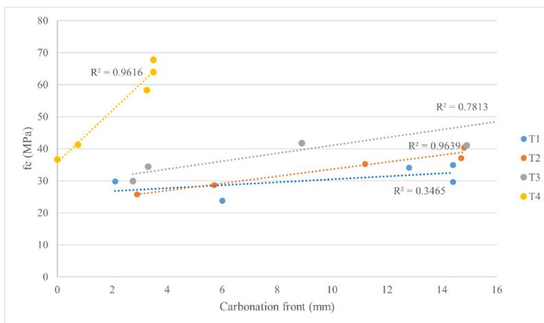
Figure 9. Compressive strength with respect to depth of carbonation depth.
