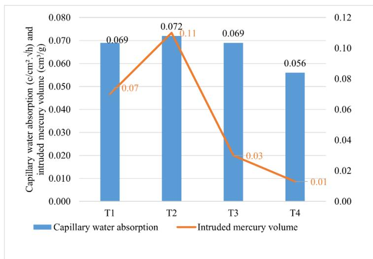
**Figure 7.** Comparison of capillary water absorption and accumulated mercury volume.
