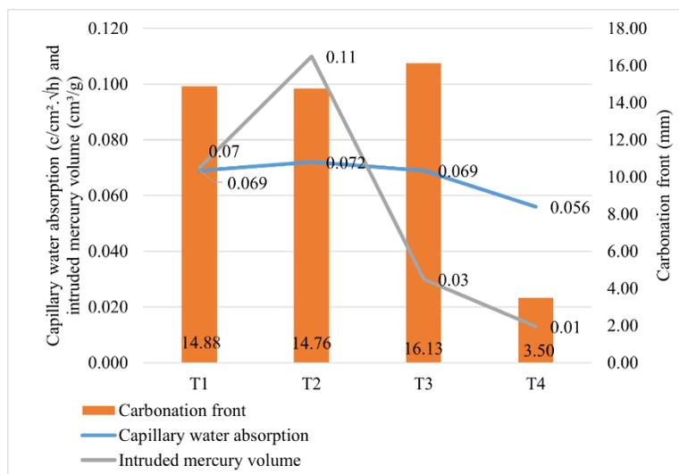
Figure 10. Comparison of capillary water absorption, intruded mercury volume and carbonation depth.
