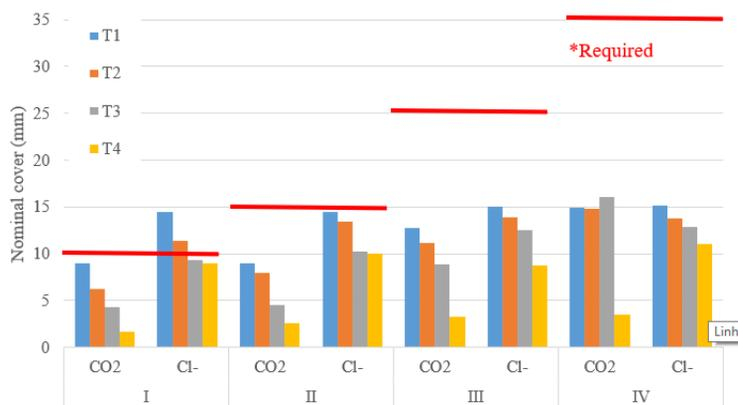
Figure 15 – Nominal cover with respect to concrete mixtures grouped by EAC.
