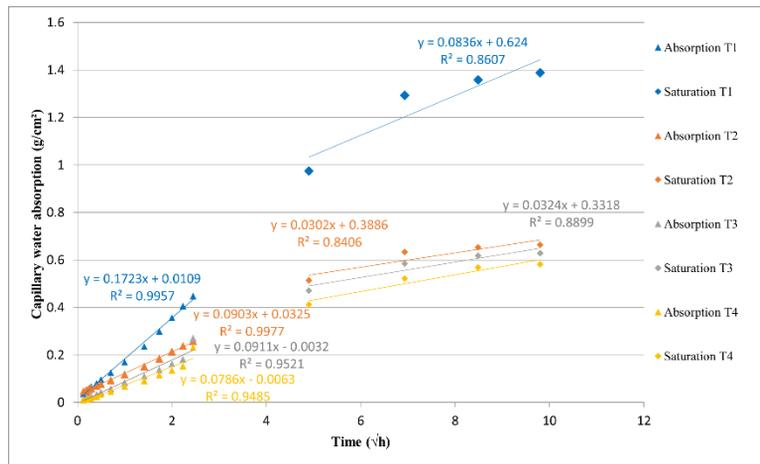
Figure 4. Capillary water absorption at 28 days for the concrete mixtures of this study.
