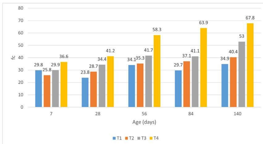
Figure 3. Potential compressive strength results for the concrete mixtures of this study.
