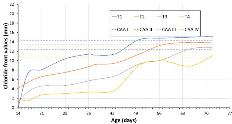
**Figure 11.** Chloride front values for the concrete mixtures of this study and EAC plateaus limits - Dashed lines present the limits from ABNT NBR 6118.
