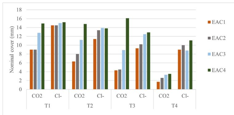
Figure 14. Nominal cover with respect to EAC grouped by concrete mixtures.
