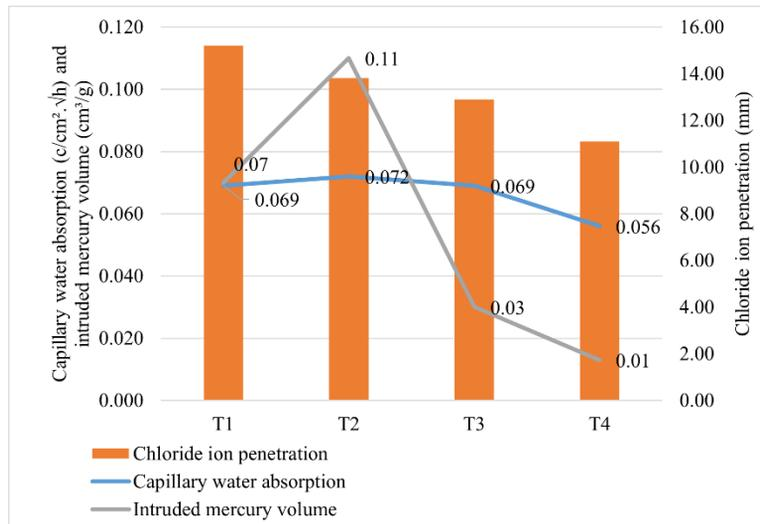
Figure 13. Comparison of capillary water absorption, intruded mercury volume and chloride ion penetration.
