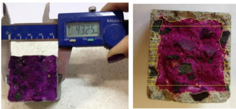
**Figure 1.** Carbonation depth mensuration with phenolphthalein solution.
