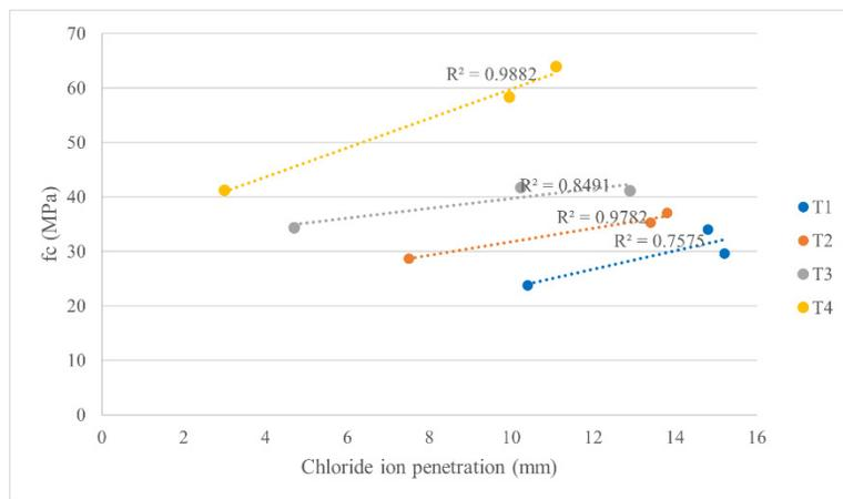
**Figure 12.** Compression strength with respect to chloride ion penetration for the concrete mixtures of this study.
