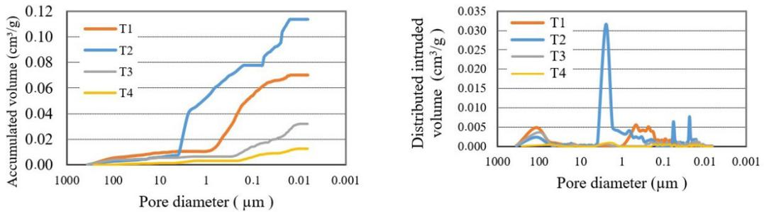
**Figure 6.** Accumulated and distributed intruded volumes from MIP with respect to pore diameter.
