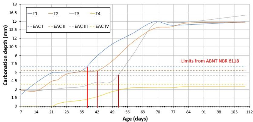
Figure 8. Carbonation depth values for the concrete mixtures of this study and EAC plateaus limits- dashed lines present the limits from ABNT NBR 6118.
