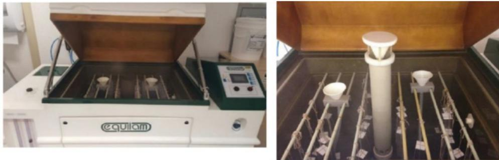
Figure 2. Salt spray chamber.
