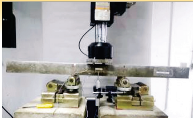
Figure 10 Beam before bending test (Author)
