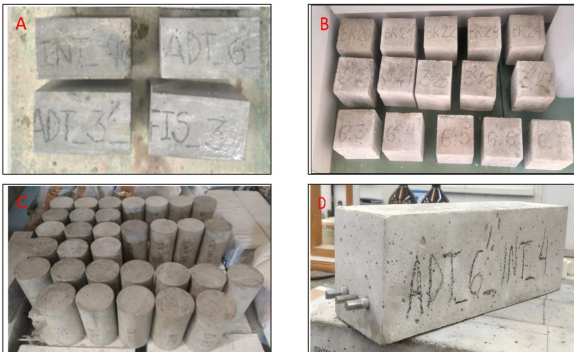
Figure 3. Illustration of the specimens: (A) prismatic; (B) cubic; (C) cylindrical; (D) Prismatics and reinforced.
