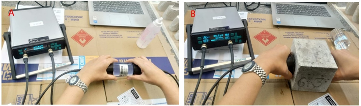
Figure 5. Equipment for UPV measurements being (A) calibrated and (B) used in the specimens.
