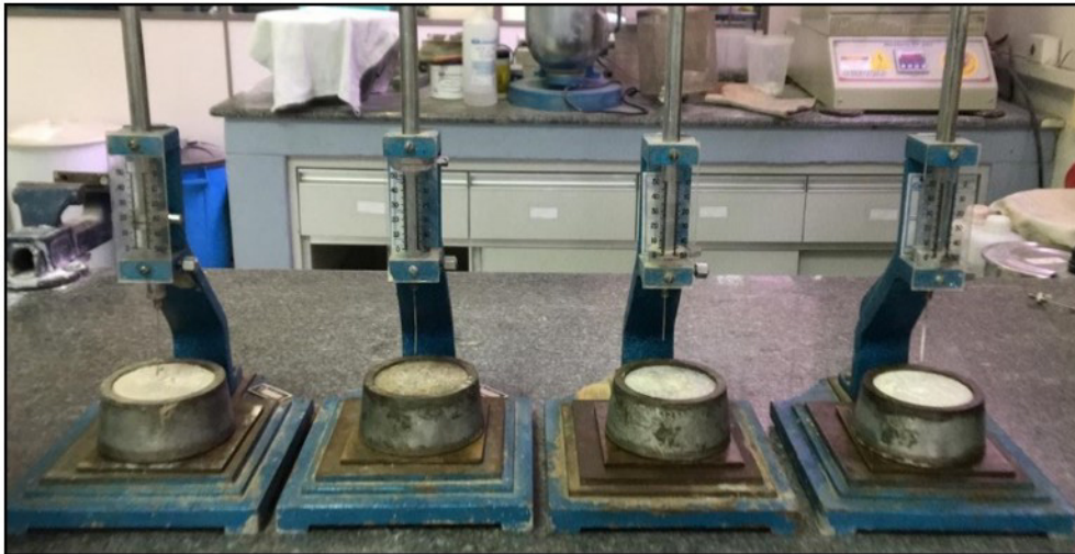
Figure 6. Setting time determination test using the Vicat apparatus.
