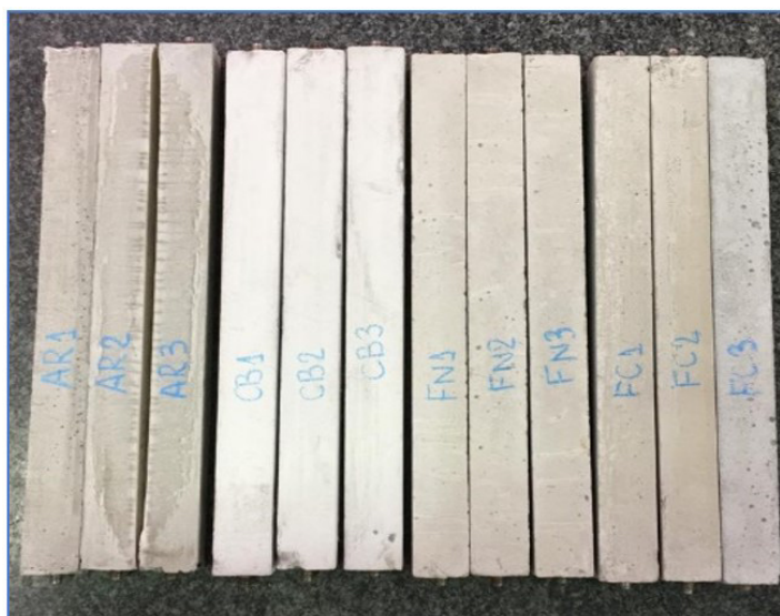
Figure 7. Test specimens from the linear shrinkage test
