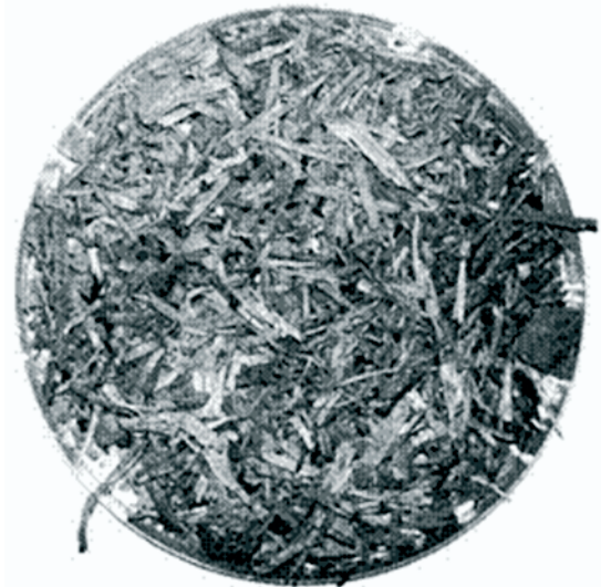
Figure 1 – Bagasse waste retained in a 2.0 mm mesh sieve
