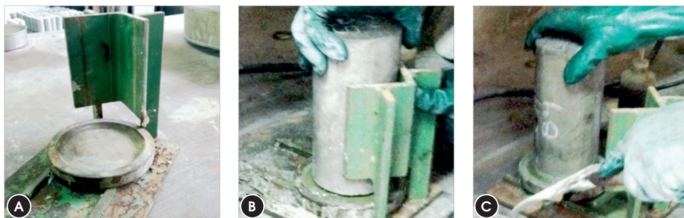
Figure 1 Alignment device used and application of sulfur mortar caps
