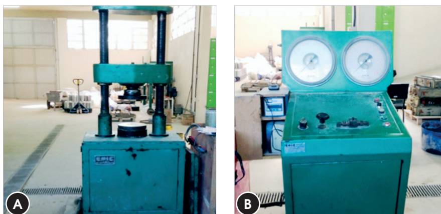
Figure 5 Compression-testing machine EMIC PCE 150 tf
