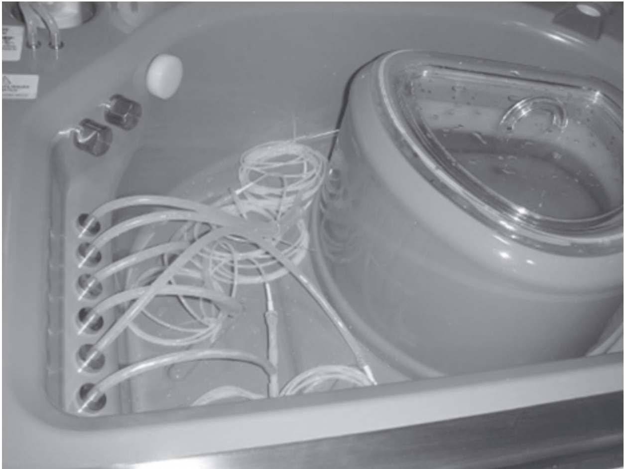
Figure 1 – Test specimens fitted into the connectors of the tested automated endoscope reprocessor.
