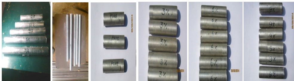
Figure 2: Cast samples of LM25-ZrO 2 composites
