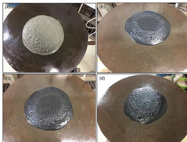
Figure 30: Determination of the consistency index (a) ACB0; (b) ACB6; (c) ACB10; (d) CBA14.
