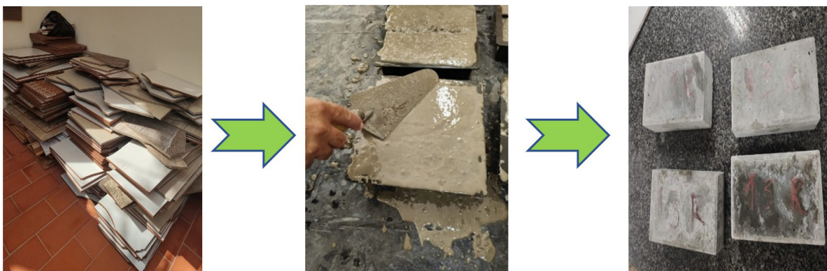
Figure 7: Production of interlocking blocks with SCC.
