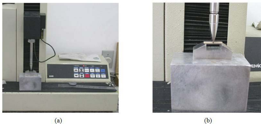
Figure 5: (a) Flexural test equipment EMIC MFDL 500. (b) Detail of the alumina bar being tested (b)
