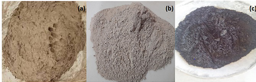
Figure 1: Raw materials used for brick manufacturing (a) clay, (b) ceramic waste powder and (c) bagasse ash.
