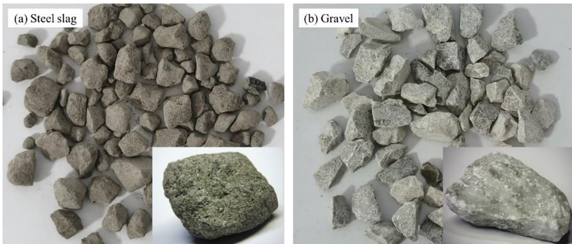
Figure 6: Morphology of SSA and limestone crushed stone.
