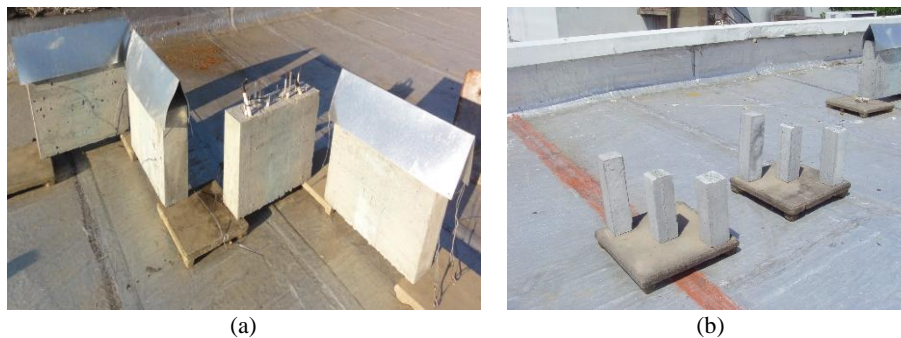
Figure 1: (a) Prototypes exposed to the external environment. (b) Specimens for carbonation tests exposed together with the prototypes showed in (a).
