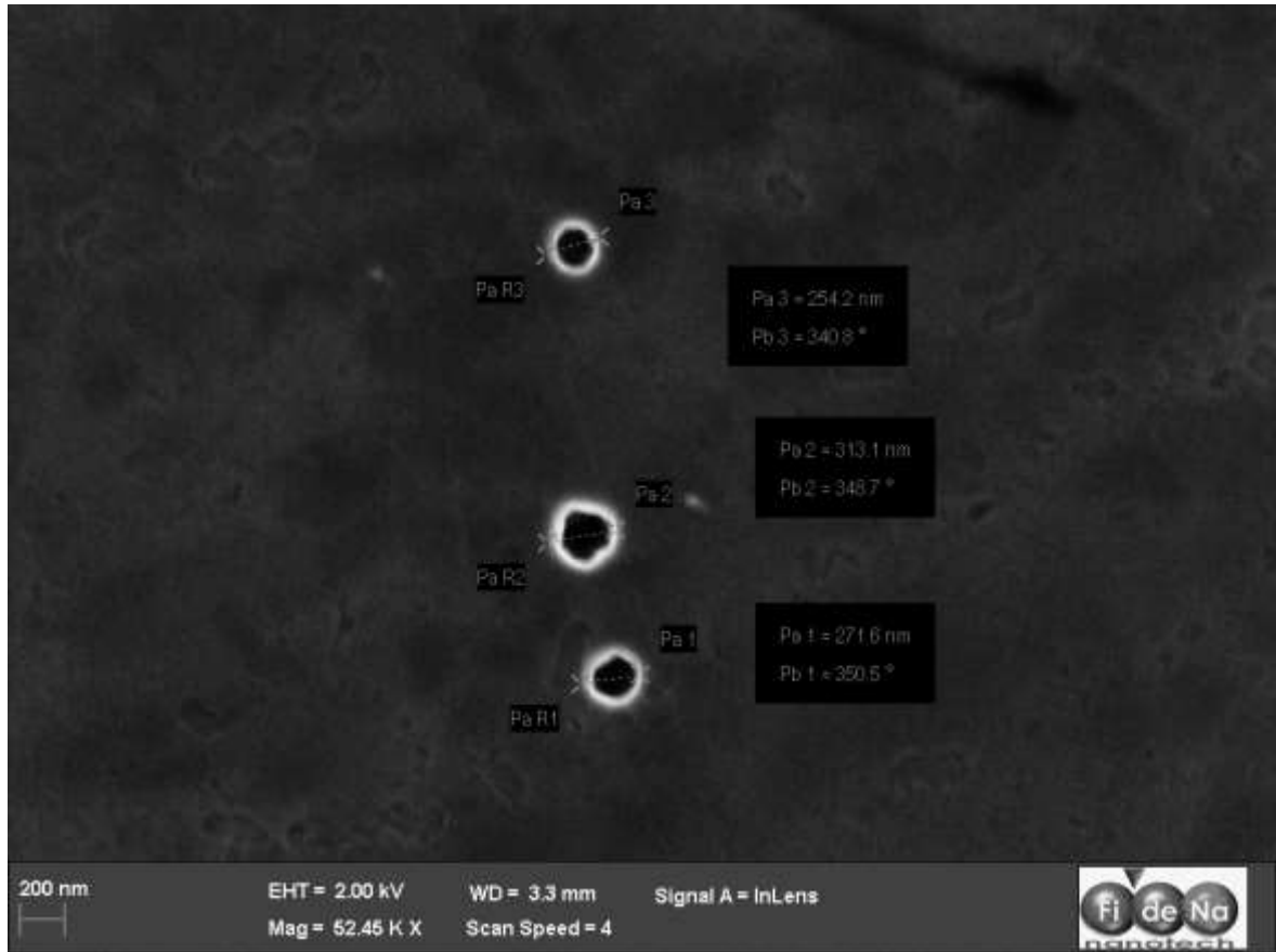
Figure 3: SEM micrograph of Mag-loaded PCL nanocapsules.
