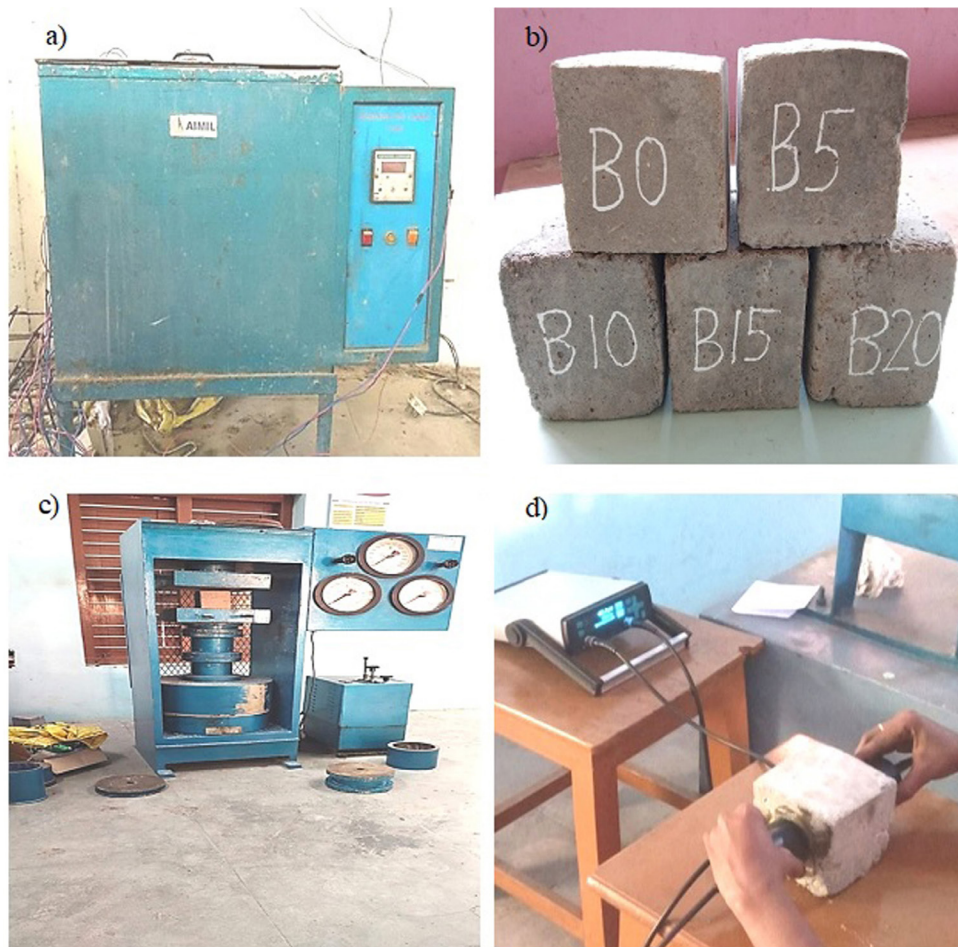
Figure 4: Photos of (a) Autoclaving machine (b) Developed samples (c) Compression testing (d) Ultrasonic pulse velocity test.
