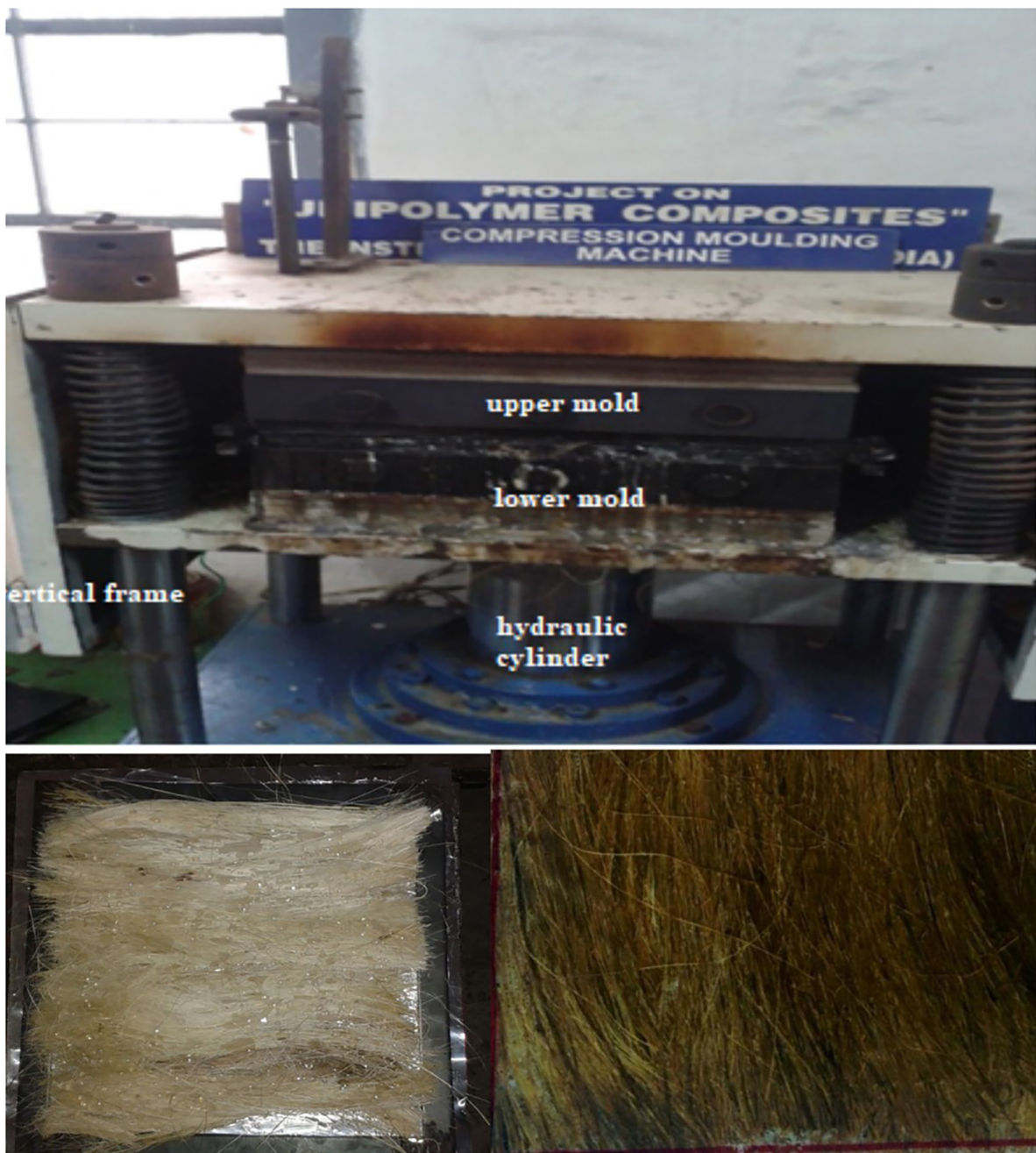
Figure 1: Experimental setup of compression molding with specimen.
