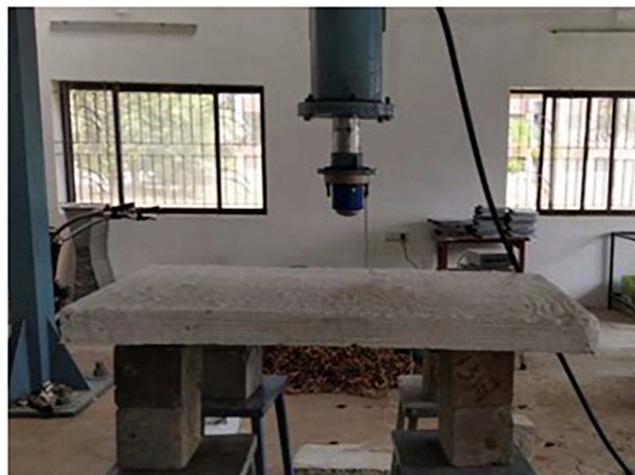
Figure 17: Cyclic load test on bamboo reinforced slab specimen.
