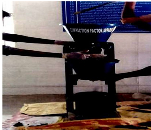
Figure 10: Compaction factor test on concrete specimens.
