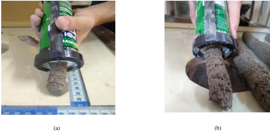
Figure 6: Extruded materials with substitution of 15% of (FA) and (MK) (a) Cementitious material with substitution of 15% (FA) without superplasticizer additive; (b) Cementitious material with substitution of 15% (MK) with 0.4% of superplasticizer additive
