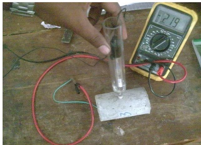
**Figure 2:** Experimental set-up for open circuit potential measurement.
