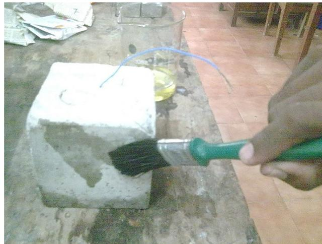
**Figure 5:** Inhibitor applied on the surface of the concrete specimen – migration process.
