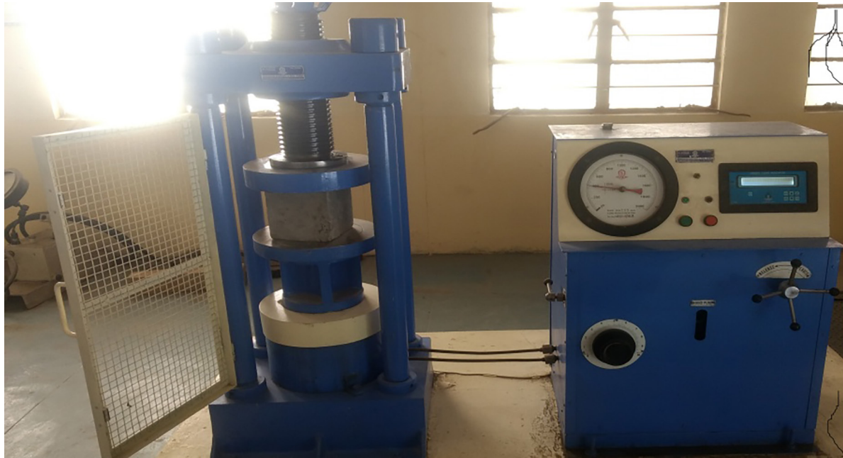
Figure 4: Compressive strength test on compression testing machine.
