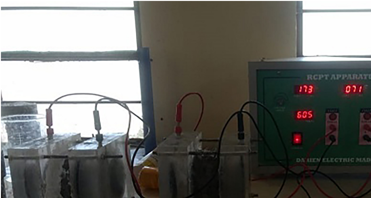
Figure 7: RCPT test process in RCPT apparatus.
