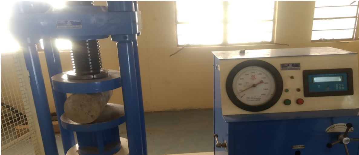
Figure 6: Split tensile strength test on compression testing machine.
