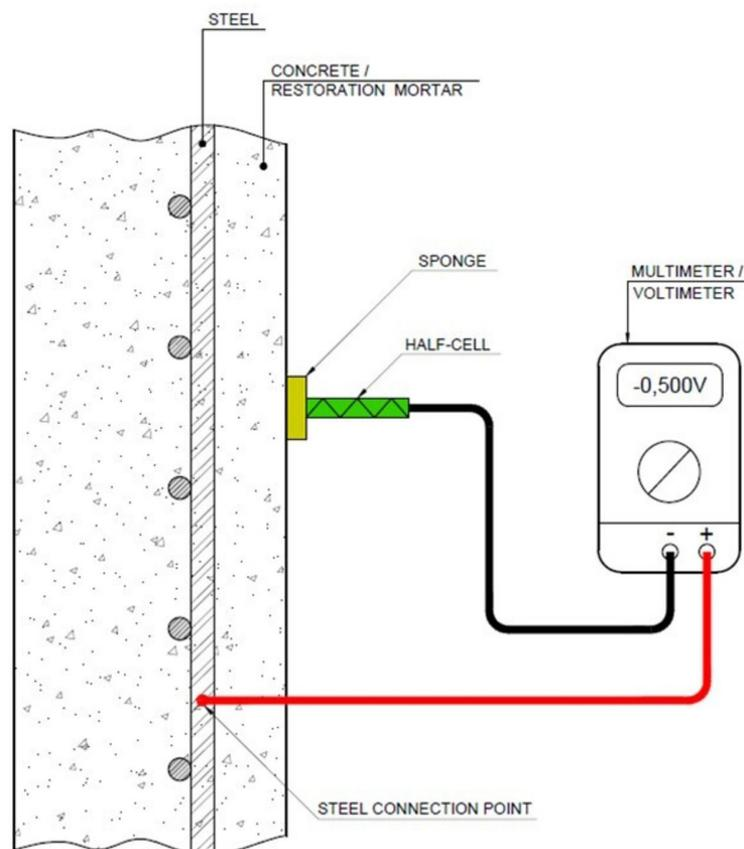
**Figure 2:** Schematic drawing on the measurement of corrosion potential. Source: the authors.
