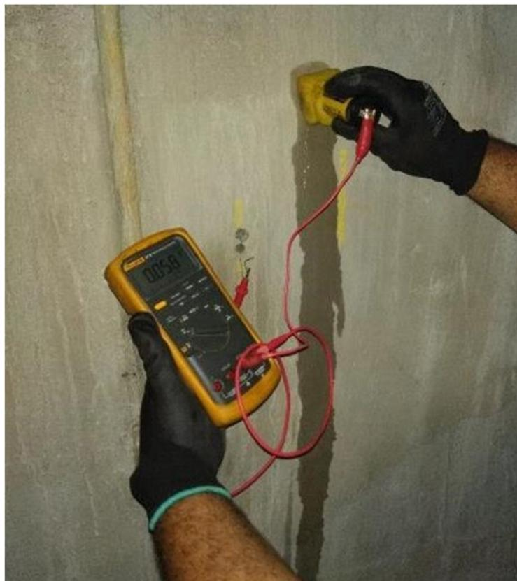
**Figure 3:** Image courtesy of IEC Engenharia, potential measurement in reinforced concrete structure. Source: IEC Engineering, 2019.
