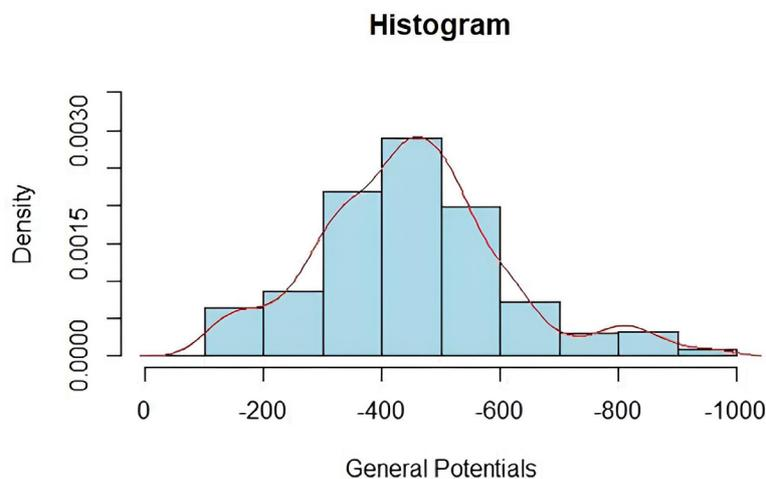
**Figure 12:** Histogram considering the electrochemical potentials of the slab studied. Source: the authors.
