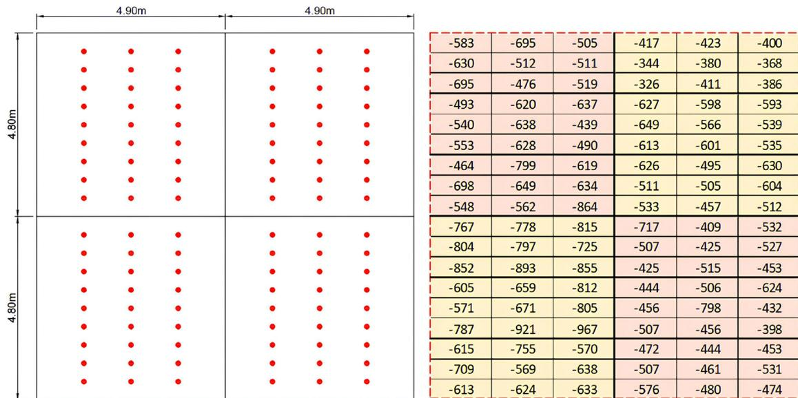
Figure 9: Reinforcement/concrete potentials of the selected slab section. Source: the authors.
