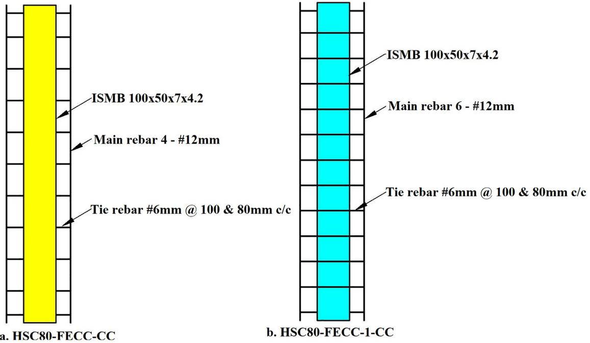
Figure 4: Reinforcement details of FECC specimen.
