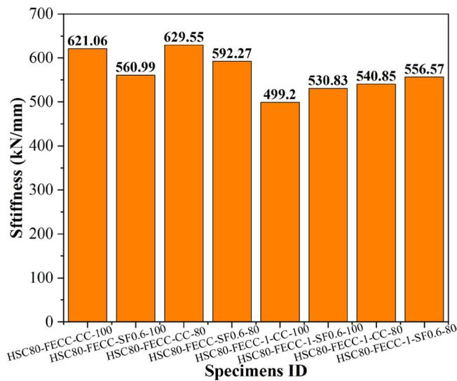
Figure 13: Stiffness of all FECC specimens.
