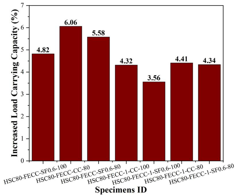
**Figure 8:** Increased load-carrying capacity of FECC specimens.
