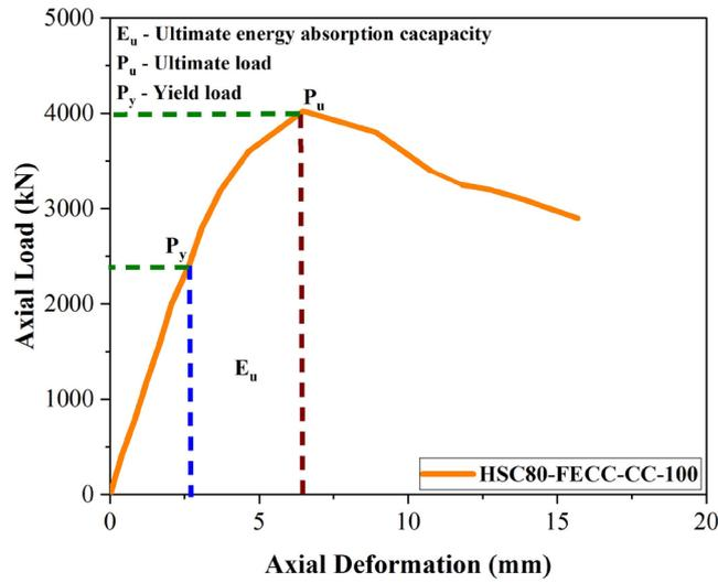
Figure 11: Model of energy absorption calculation of FECCs.
