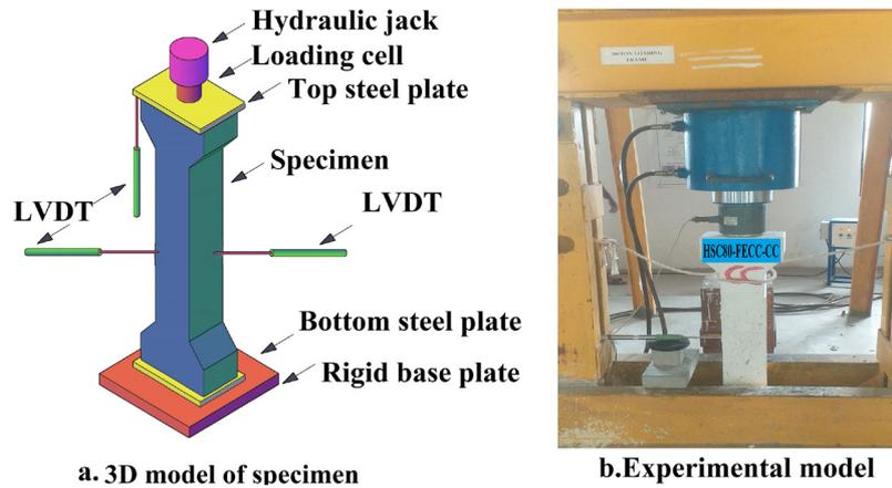
Figure 6: Experimental setup of the specimen.
