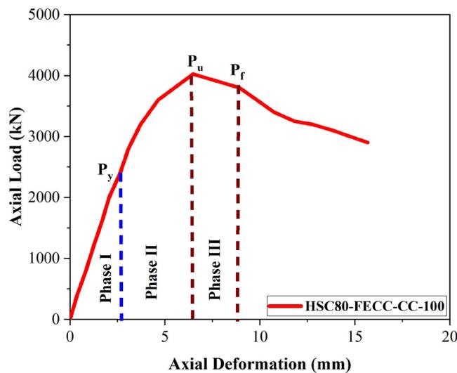
**Figure 9:** Model of ductility calculation of FECC.
