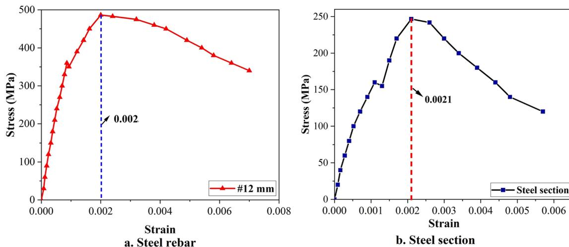
**Figure 2:** Stress-strain curve for steel rebar and section.
