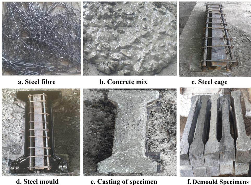
Figure 5: Fabrication of FECC specimens.
