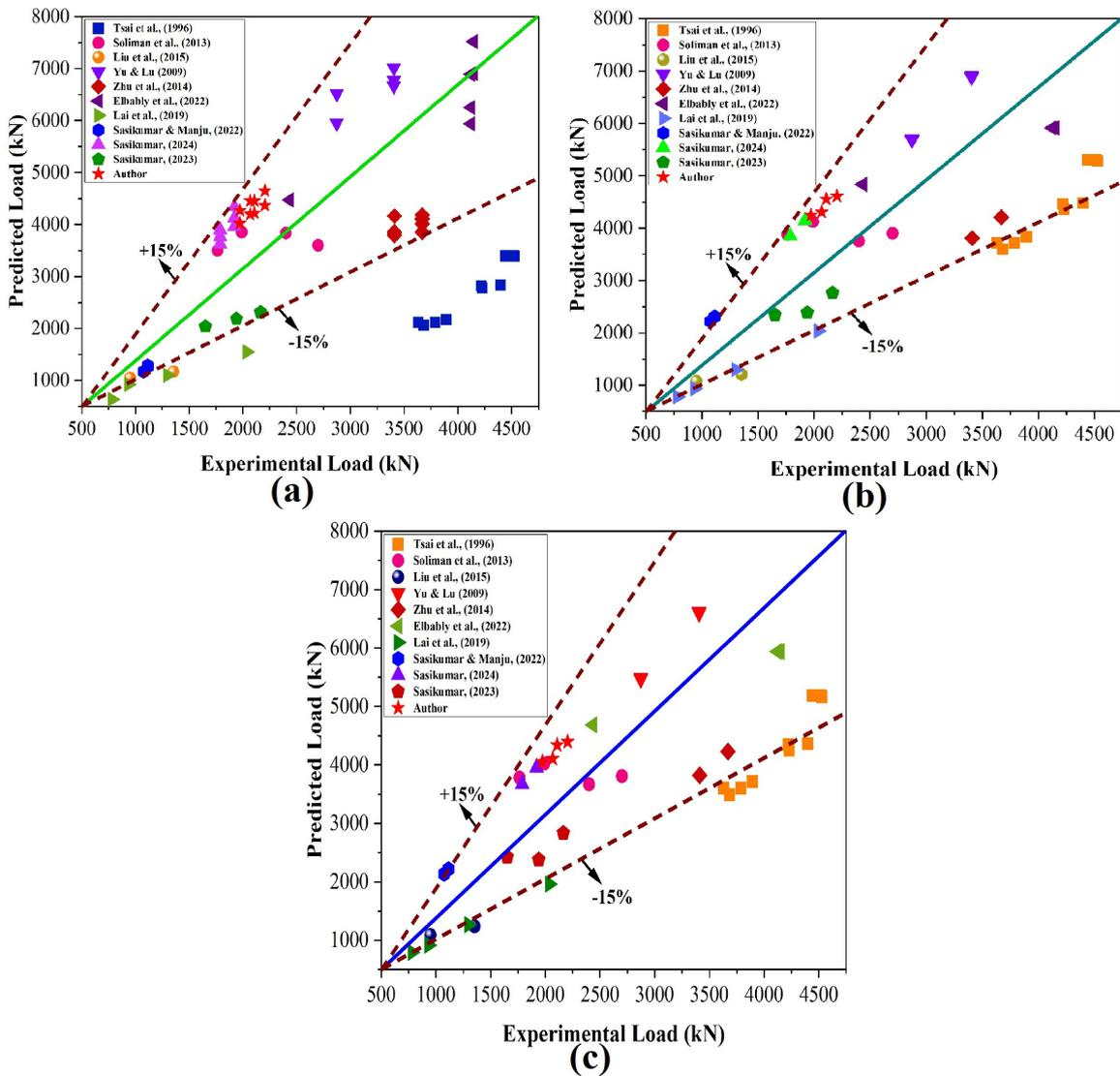
**Figure 15:** Comparative study between experimental and predicted results from literature studies. (a) IS prediction; (b) JGJ prediction; (c) EC4 prediction.
