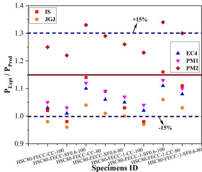
**Figure 17:** Reliability of experimental and analytical results of FECC specimens.
