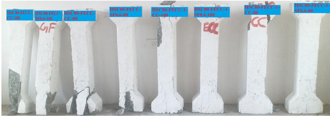
**Figure 14:** Failed FECC specimens.
