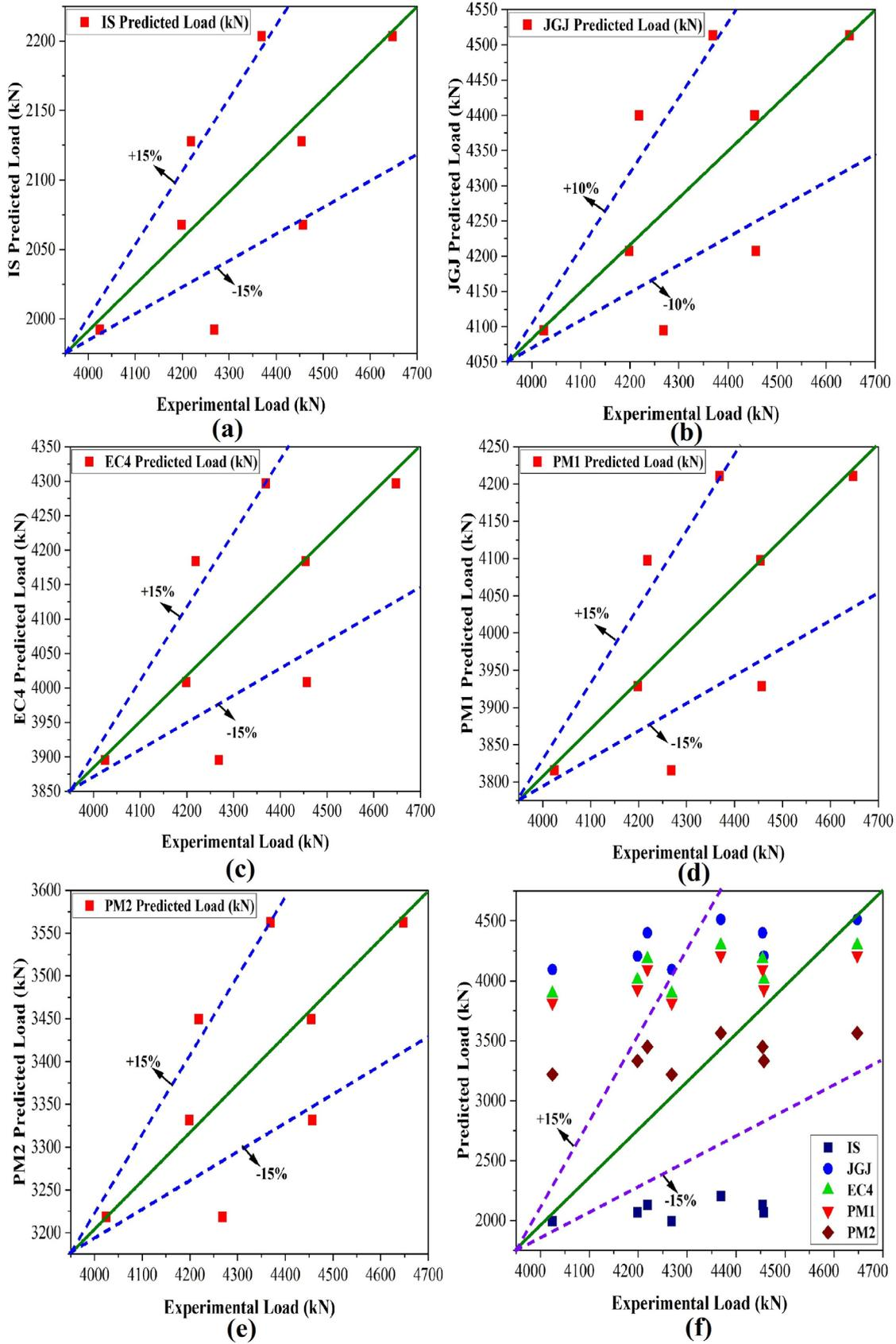
Figure 16: Comparison between experimental and predicted results for various codes and proposed methods. (a) IS prediction; (b) JGJ prediction; (c) EC4 prediction; (d) PM1 prediction; (e) PM2 prediction; (f) overall prediction.
