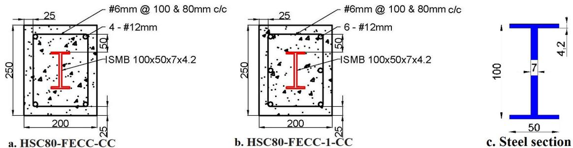
**Figure 3:** Cross-section details of the column specimens and steel section.
