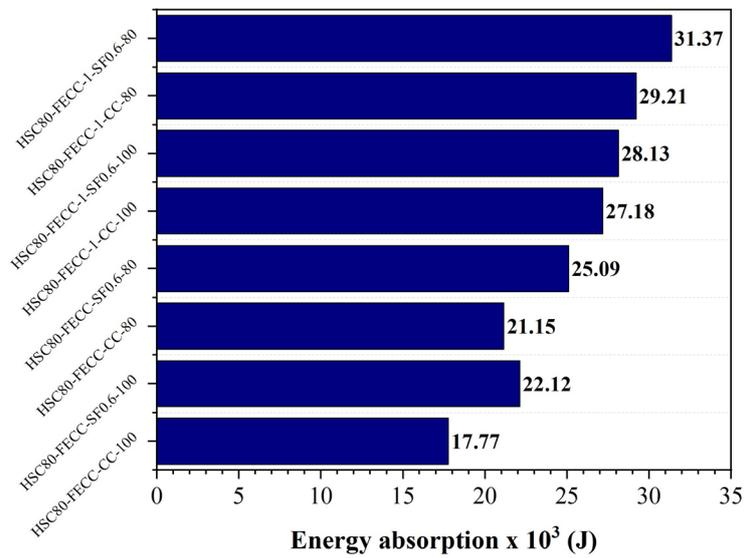
Figure 12: Energy absorption capacity of all FECC.
