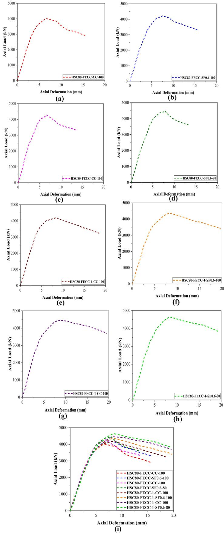
**Figure 7:** Experimental axial load versus deformation of column specimens. (a) HSC80-FECC-CC-100; (b) HSC80-FECC-SF0.6-100; (c) HSC80-FECC-CC-80; (d) HSC80-FECC-SF0.6-80; (e) HSC80-FECC-1-CC-100; (f) HSC80-FECC-1-SF0.6-100; (g) HSC80-FECC-1-CC-100; (h) HSC80-FECC-1-SF0.6-80; (i) All groups of FECC specimens.
