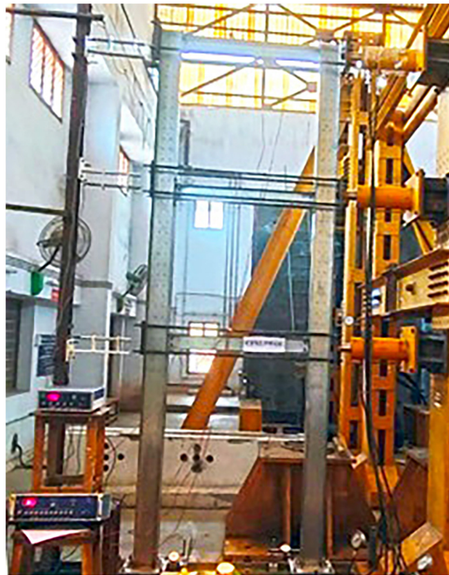
Figure 4: Experiment test setup for test specimen (Ex. CFSF2WL).
