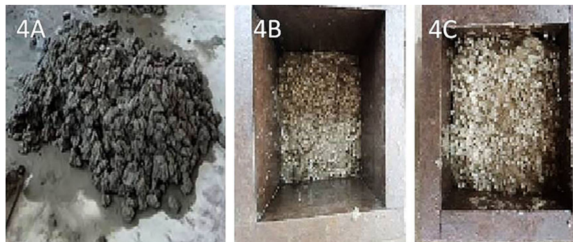
Figure 4: (a), (b) and (c) Incorporation of beads in concrete specimen.
