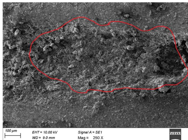
Figure 11: Traces of friction material on the brake disc surface.
