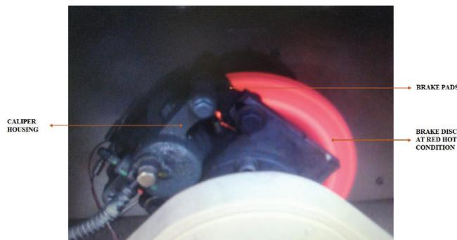
Figure 6: Red hot condition of brake disc during wear test.
