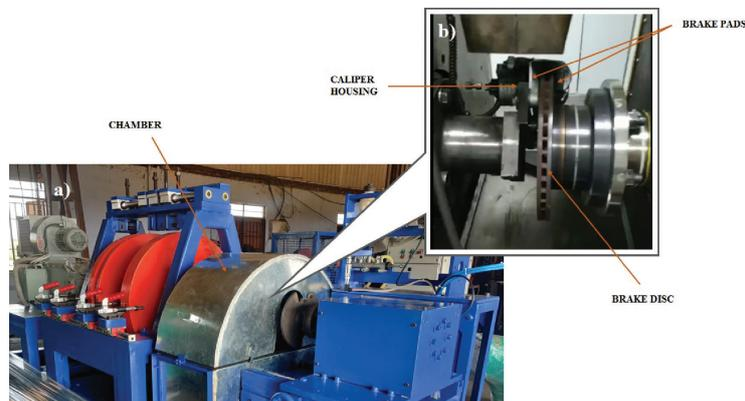
**Figure 2:** (a) Full-scale inertia brake dynamometer test setup (b) Brake disc assembly.
