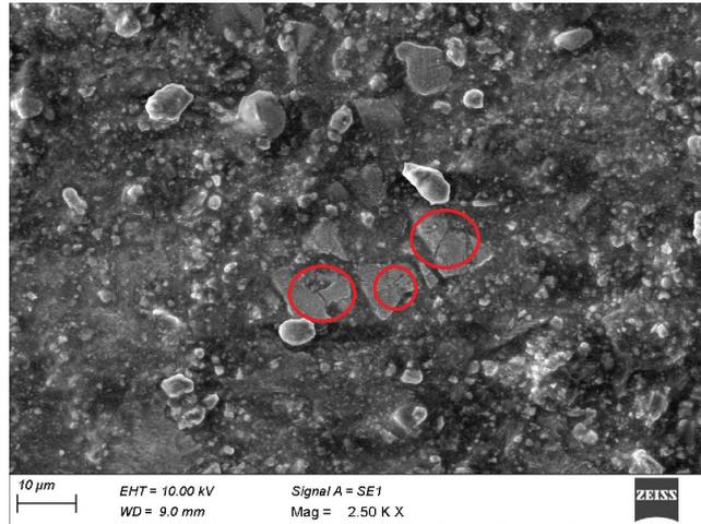
Figure 12: Cracks on the surface of the brake disc.
