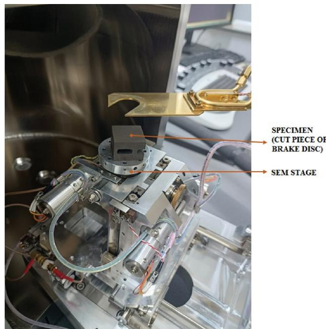
Figure 10: The specimen under metallography testing.
