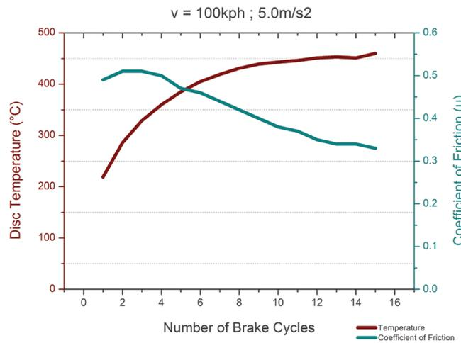
**Figure 4:** Influence of temperature on friction during second fade sequence.
