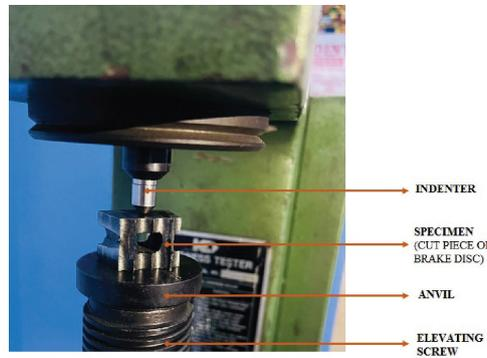
Figure 13: Hardness testing of the specimen.
