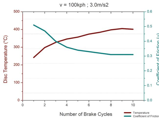
**Figure 3:** Influence of temperature on friction during first fade sequence.
