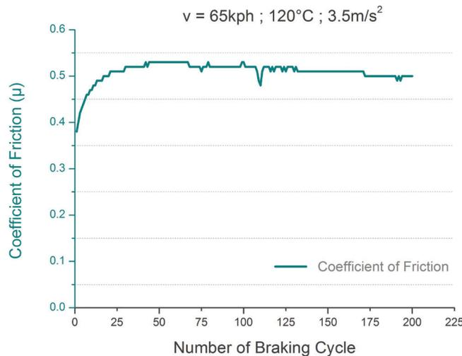
Figure 7: Influence of the number of braking cycles on friction.
