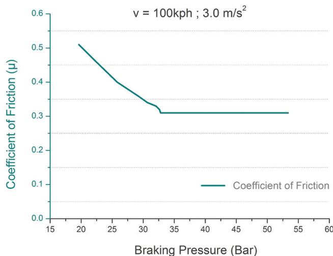
Figure 8: Influence of braking pressure on friction.
