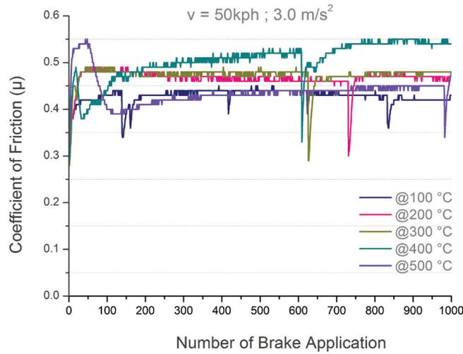
Figure 5: Influence of temperature on friction during the wear test.
