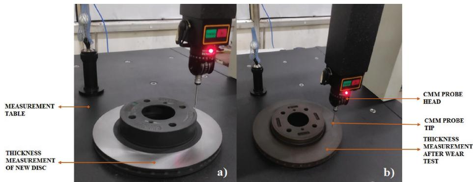
**Figure 9:** (a) Thickness measurement of new disc in CMM (b) Thickness measurement after wear test.
