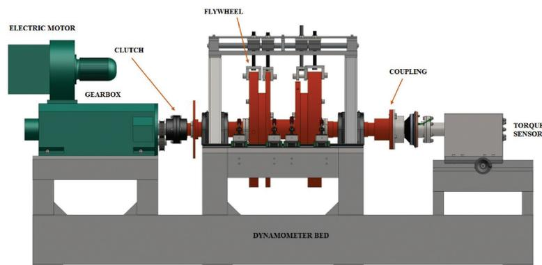
**Figure 1:** Schematic of inertia brake dynamometer.
