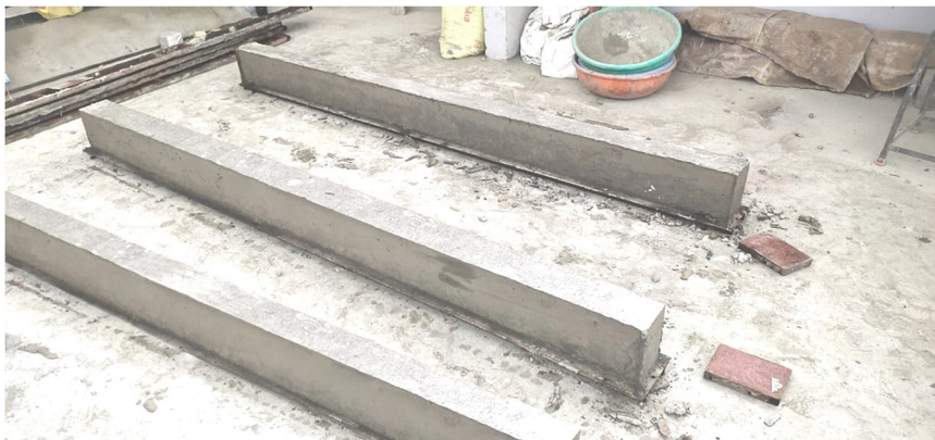
Figure 3: Casting of RC beam specimens.
