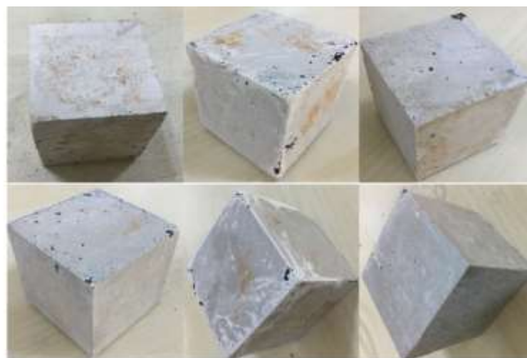
Figure 2: Hardened MK, MKC05, MKC10, MKC15, MKC20, MKC25 specimens, respectively
