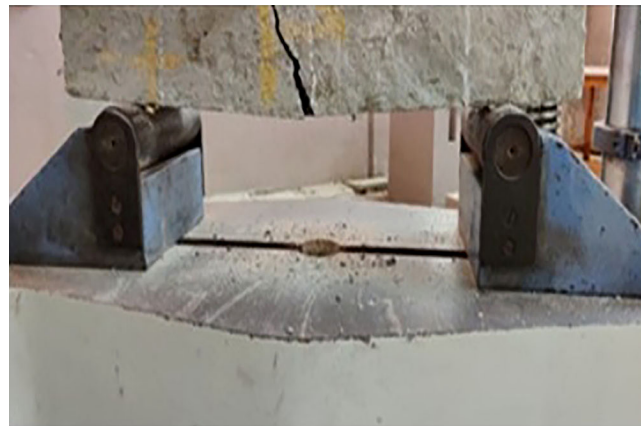
Figure 7: Jute-fiber mixed in concrete specimen.
