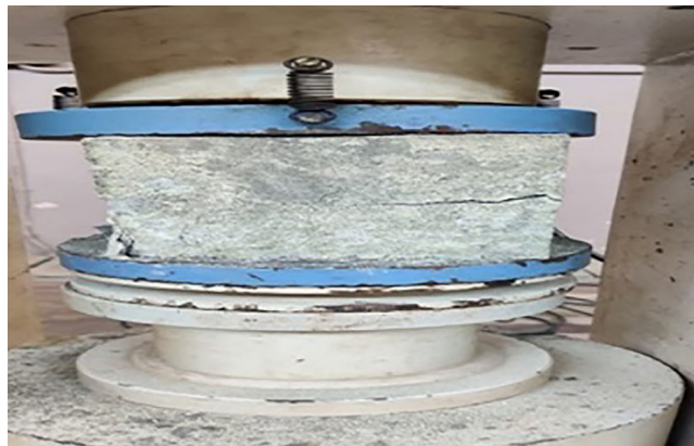
Figure 4: Failure of cube specimen under compression.
