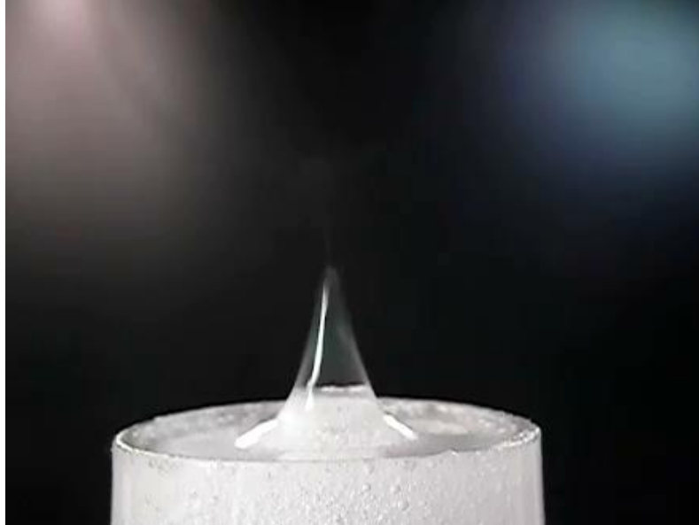
Figure 17: A polymer bubble in presence of an electrostatic field
