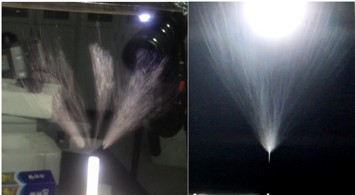
Figure 5: Multiple charged jets from a broken bubble.
