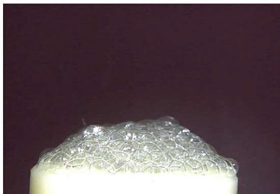
Figure 22: Multiple bubble electrospinning. Larger bubbles cannot be used for fiber fabrication
