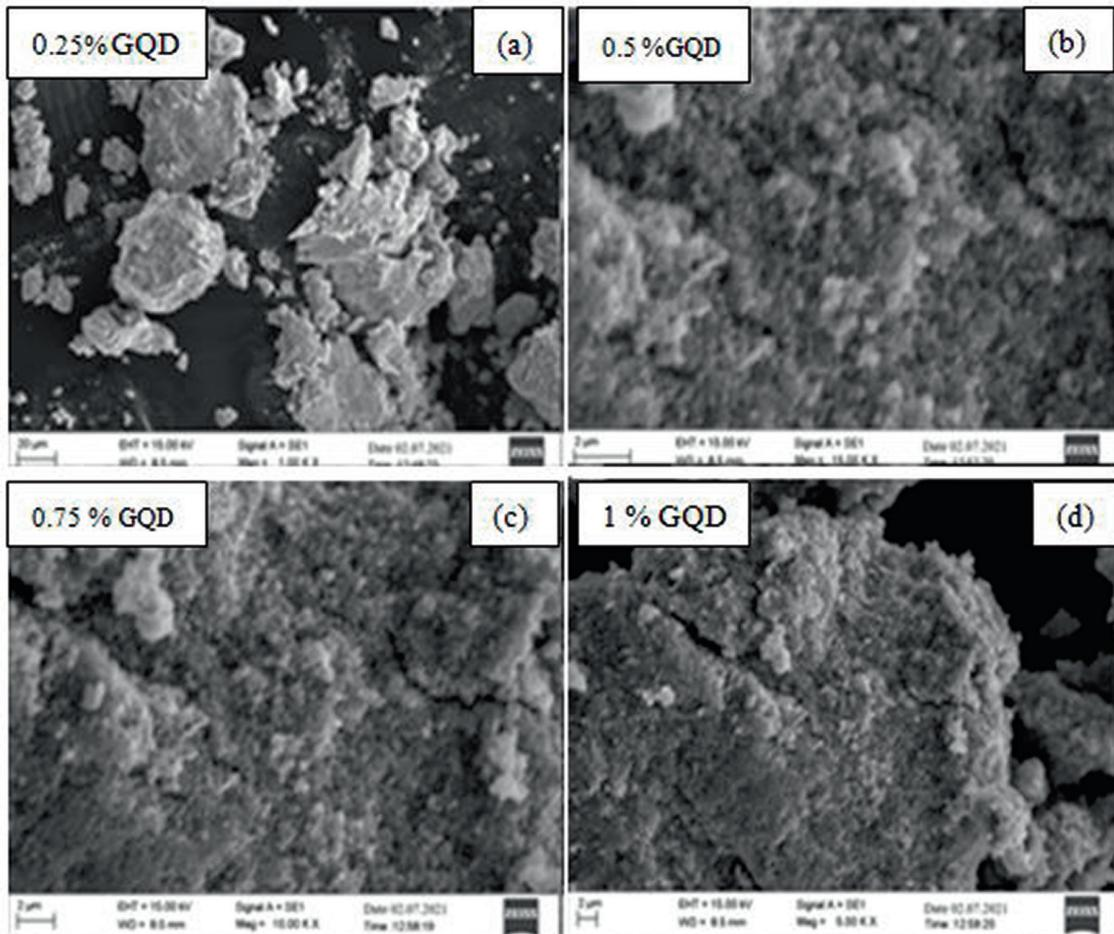
Figure 6: SEM images of cube shaped Aluminum 2024 metal matrix composites.
