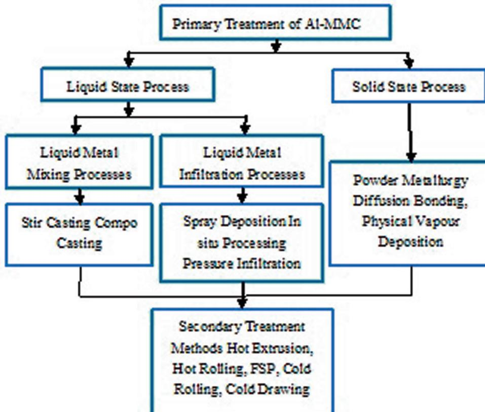
Figure 1: Primary and secondary treatment method of Al-MMC.
