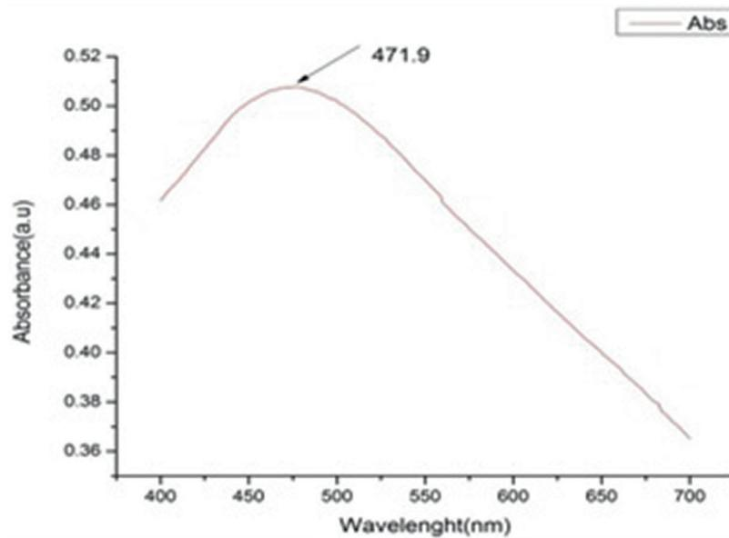
Figure 2: UV absorption spectra of Aluminum 2024 metal matrix.
