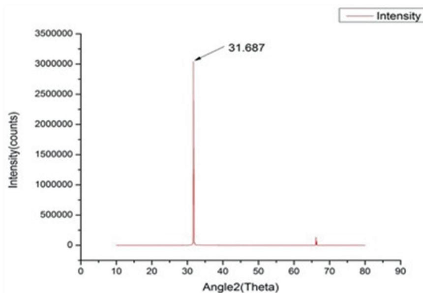
Figure 3: XRD analysis of Aluminum 2024 metal matrix.
