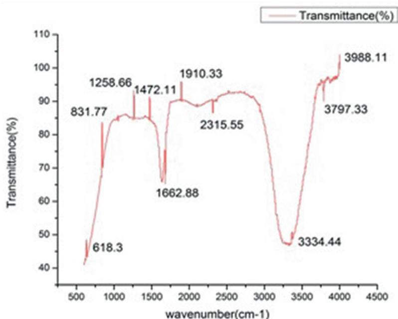
**Figure 4:** FTIR signals of Aluminum 2024 metal matrix composites.
