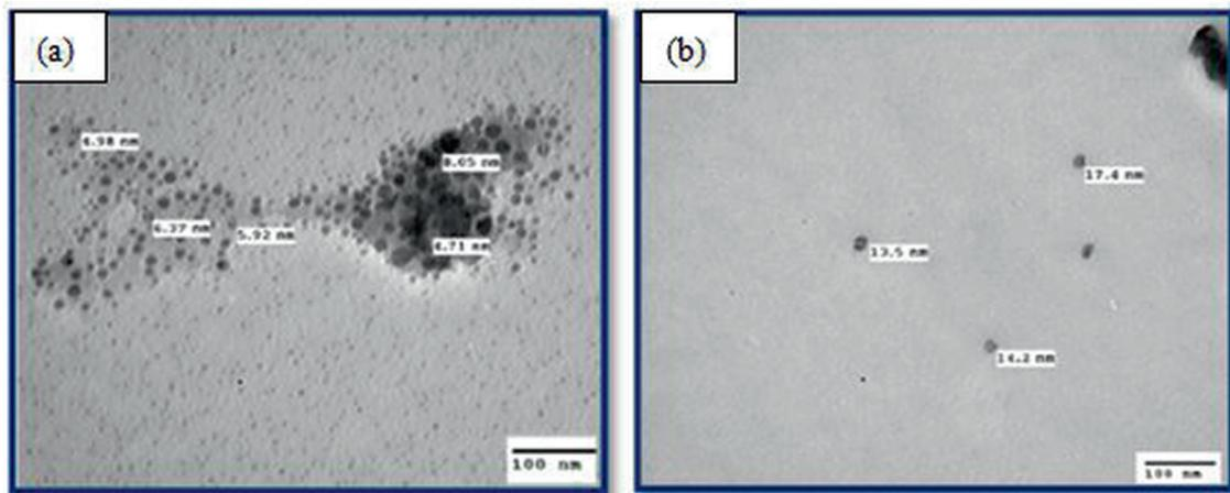
Figure 7: Aluminum 2024 in (a) TEM image with semi-spherical and spherical forms (b) Metal matrix's nanoscale size.
