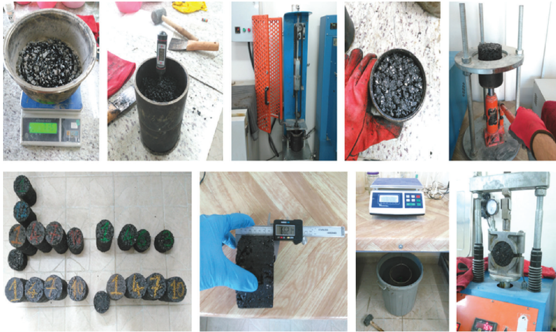
Figure 3: Marshall test steps of SMA samples.
