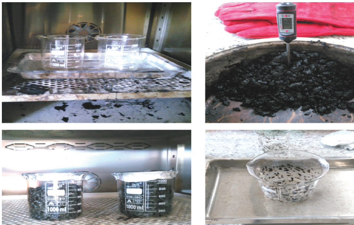
Figure 4: Preparation SMA mixture samples for the Schellenberg test.
