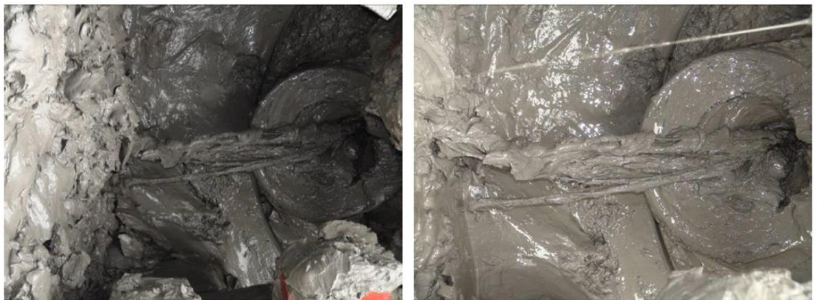
**Figure 4:** PVD blockage of sludge tank.
