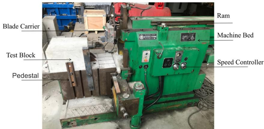
Figure 13: Linear cutting test device.
