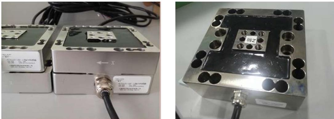
Figure 14: Triaxial force sensors.
