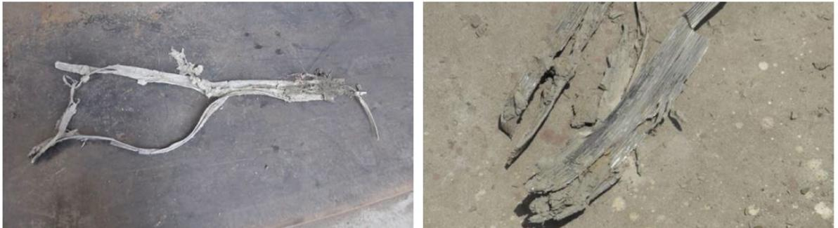
**Figure 3:** Cutting chips from PVD with ripper.
