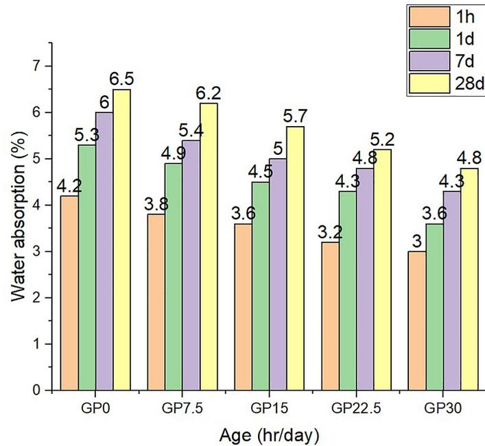
**Figure 4:** Water absorption of SCC in different time periods.
