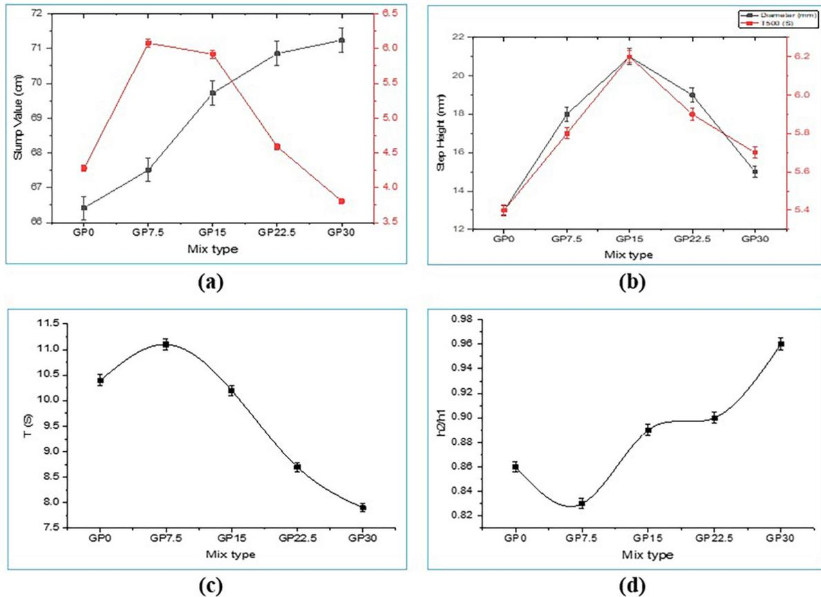
**Figure 2:** Tests on fresh concrete (a) Slump Value, (b) J – ring, (c) V – funnel and (d) L-box respectively.
