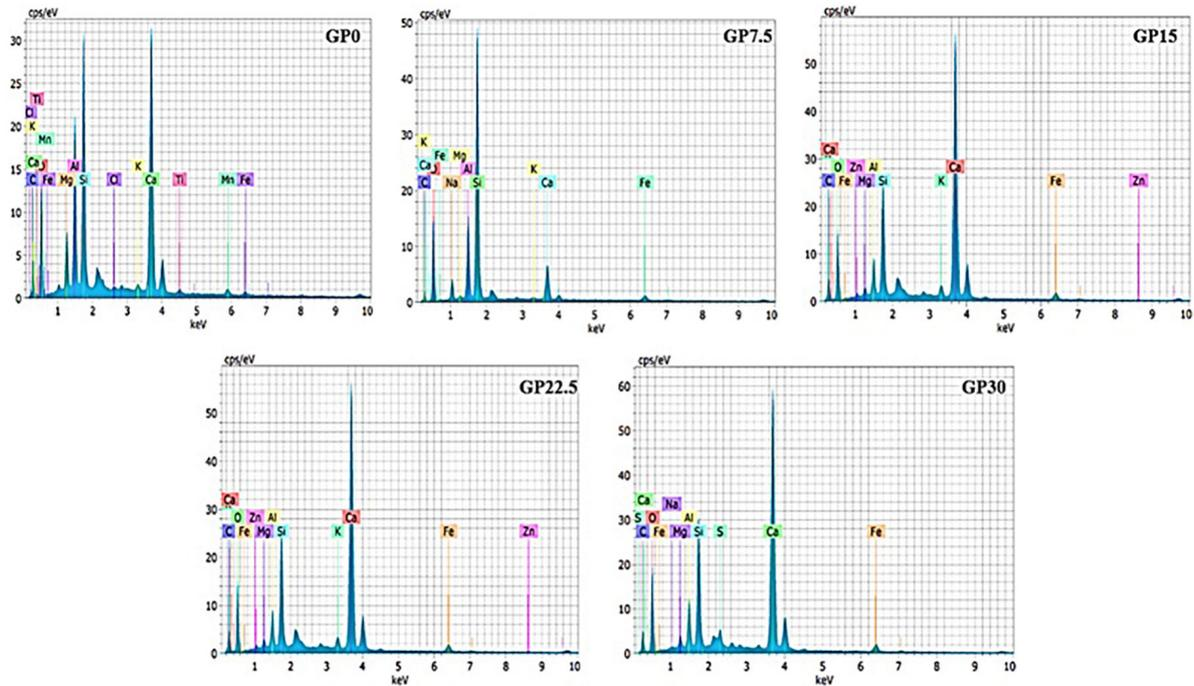
**Figure 8:** EDX images of concrete (SCC) mixes with different mix proportions.
