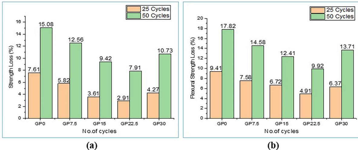
Figure 6: (a) Changes in compressive strength and (b) Changes in flexural strength after free-thaw cycles.
