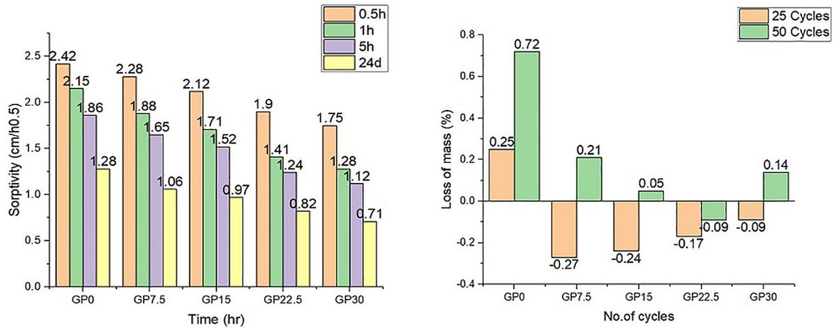
Figure 5: (a) SCC capillary water absorption and (b) Changes in weight mass after freeze and thaw cycles.
