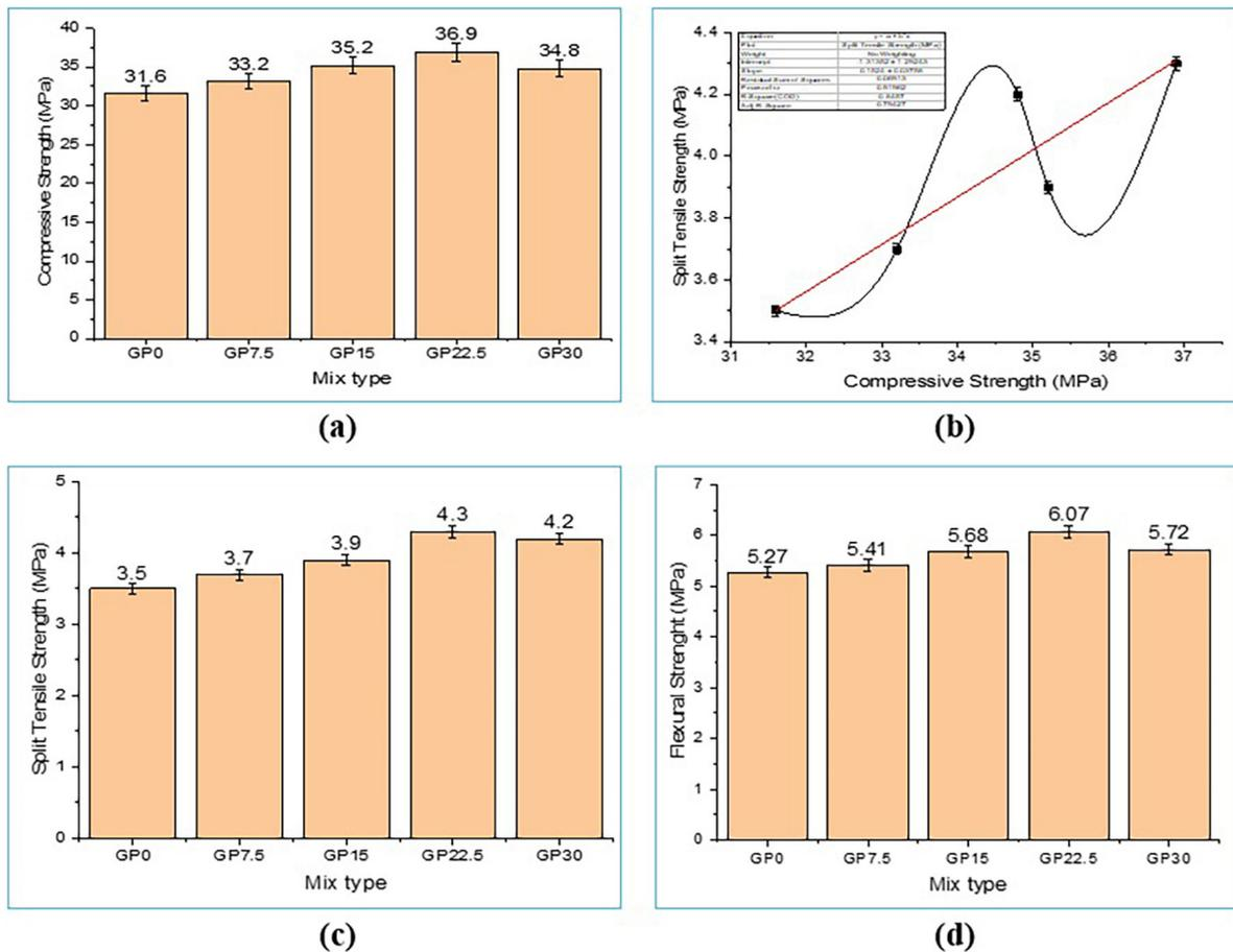
**Figure 3:** (a) Compressive strength, (b) Split tensile vs compressive strength, (c) Split tensile and (d) Flexural strength of self-compacting concrete mixes.
