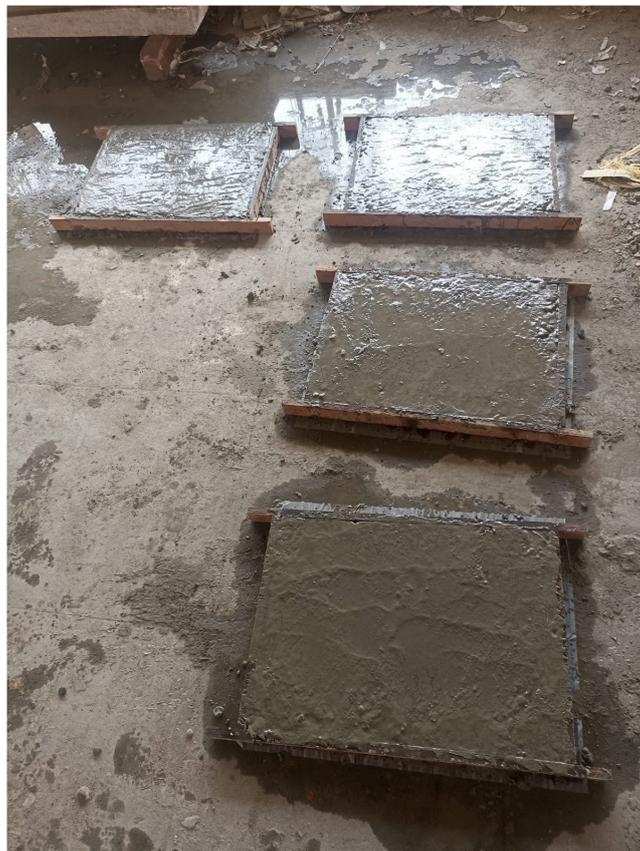
Figure 2: Casting of specimens.
