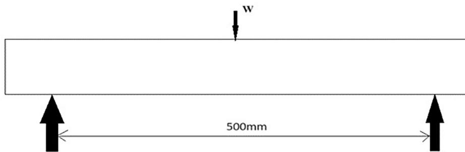
Figure 10: Schematic representation of supporting condition of slab.
