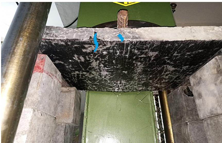
**Figure 18:** Failure mode of fire damaged GPC slabs wrapping with BFRP laminates.
