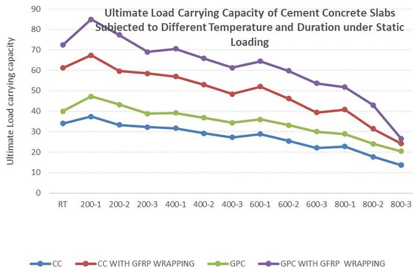
**Figure 14:** Overall comparison of Ultimate load carrying capacity of Cement and Geopolymer slabs at various temperatures and various durations.
