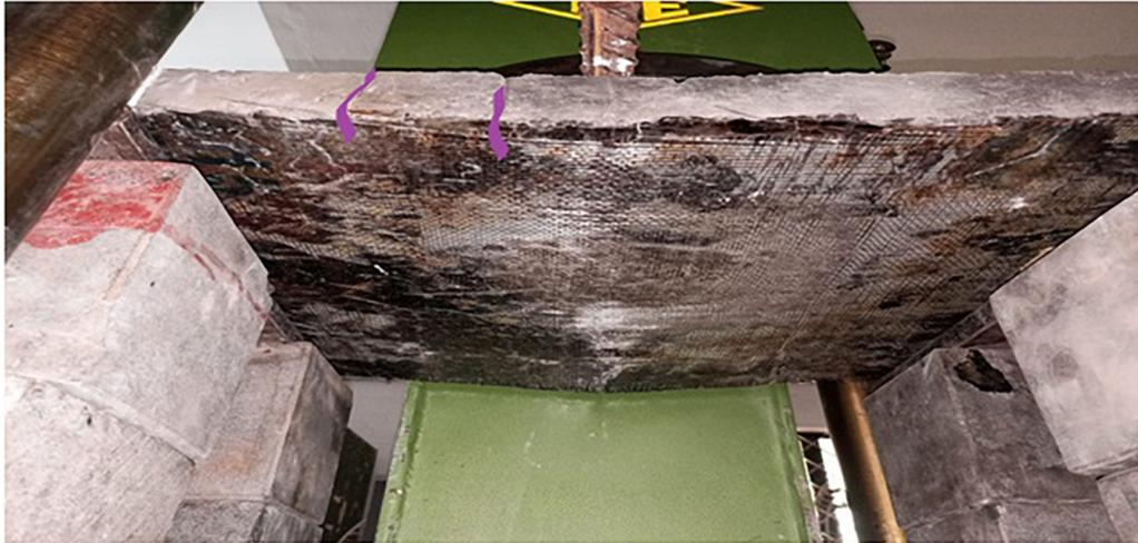
**Figure 16:** Failure mode of fire damaged geopolymer concrete slab.
