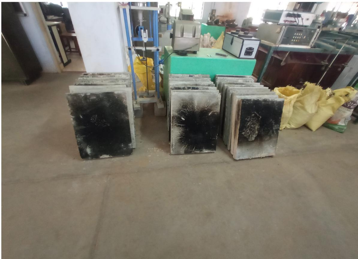
**Figure 8:** Fire damaged slabs.
