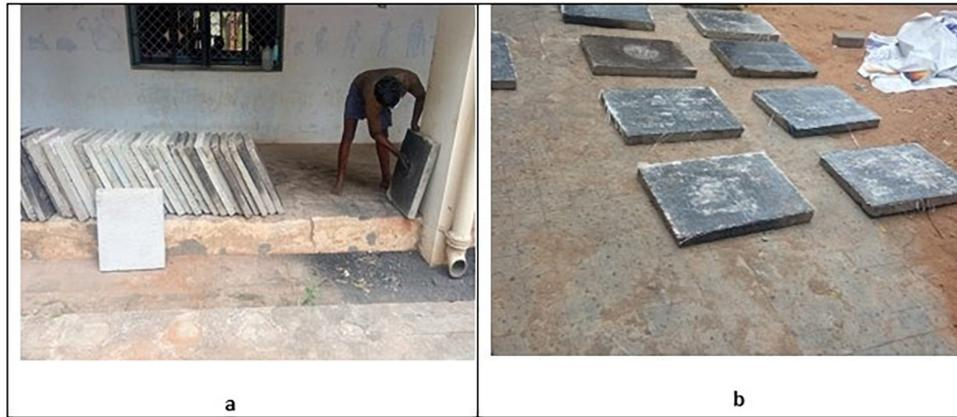
Figure 9: a) Surface cleaning process. b) Slab wrapped with BFRP laminates.
