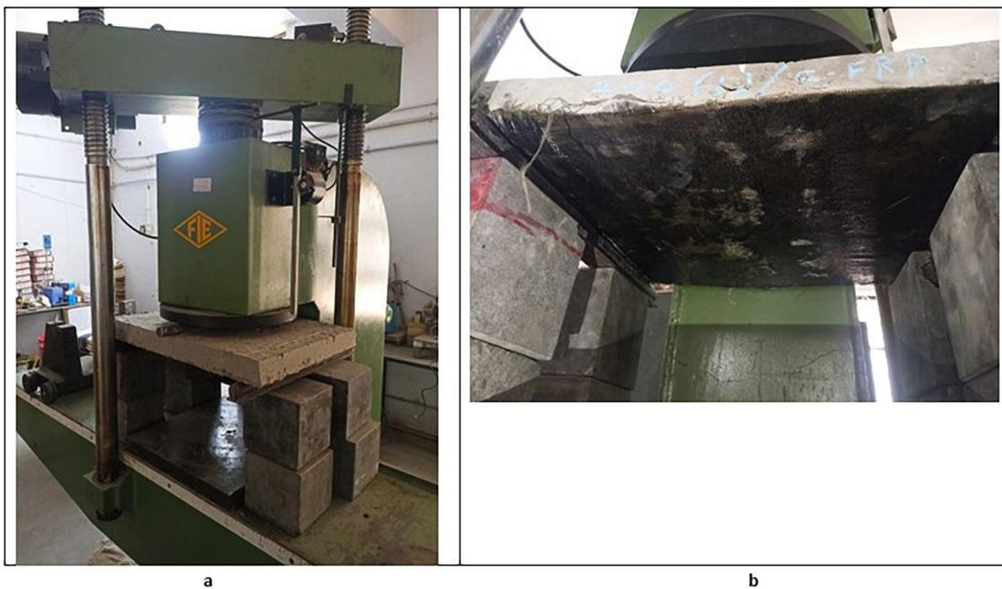
Figure 11: a) Testing of fire damaged slab without wrapping. b) Testing of fire damaged slab retrofitted with BFRP laminates.
