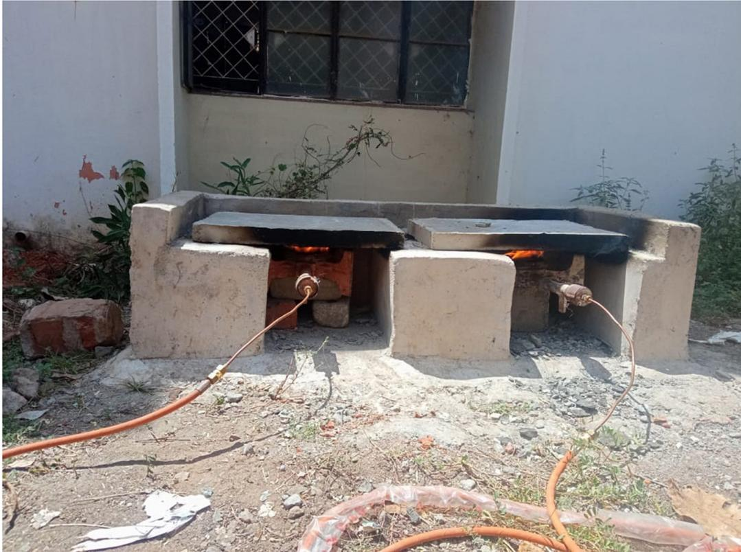
**Figure 7:** Exposure of fire on concrete slab.
