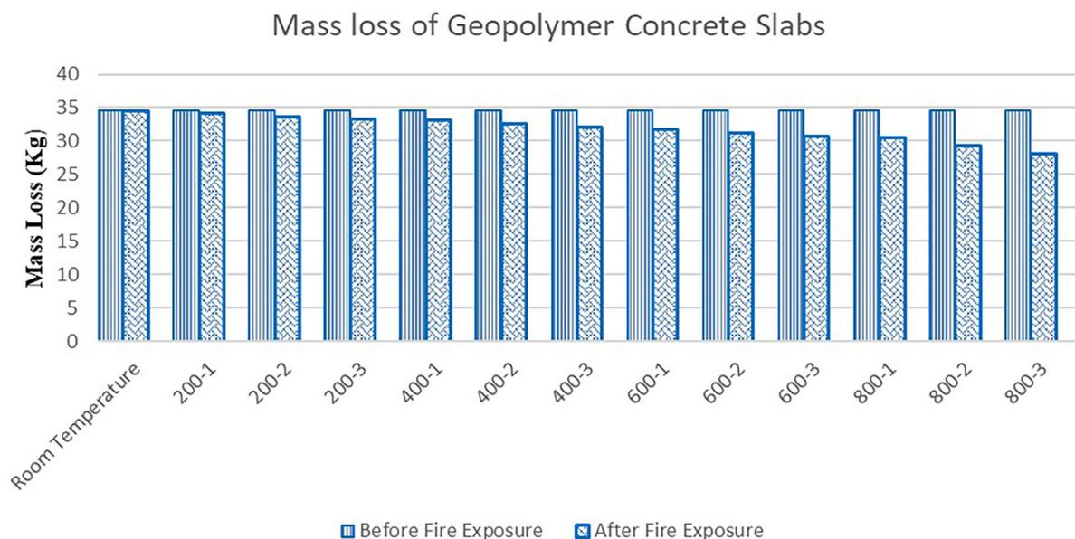
Figure 13: Mass loss of geopolymer concrete slabs subjected to different temperature and duration.
