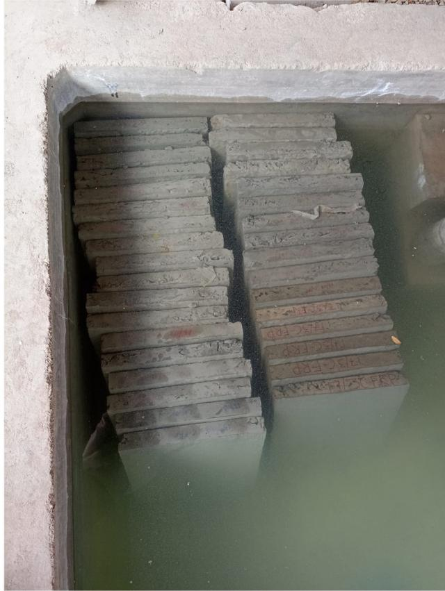
Figure 3: Water curing of cement concrete slabs.
