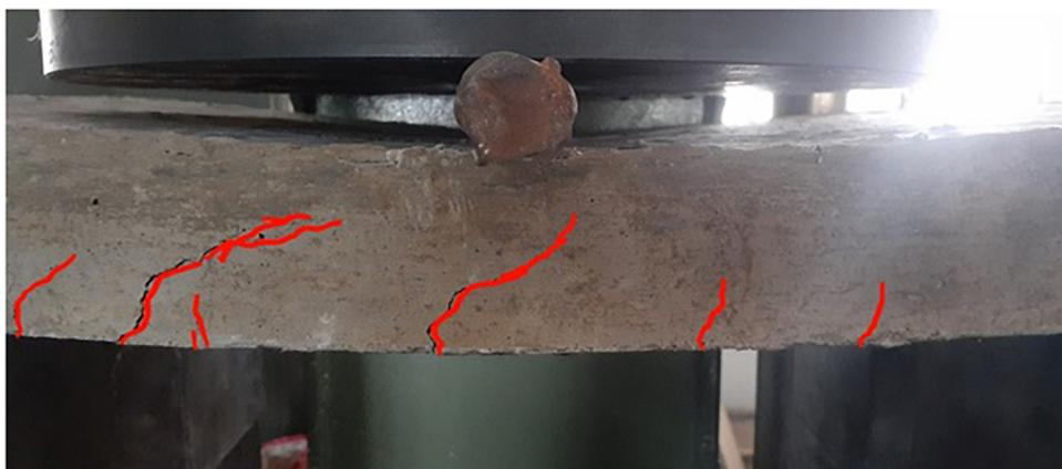
**Figure 15:** Failure mode of fire damaged cement concrete slab.
