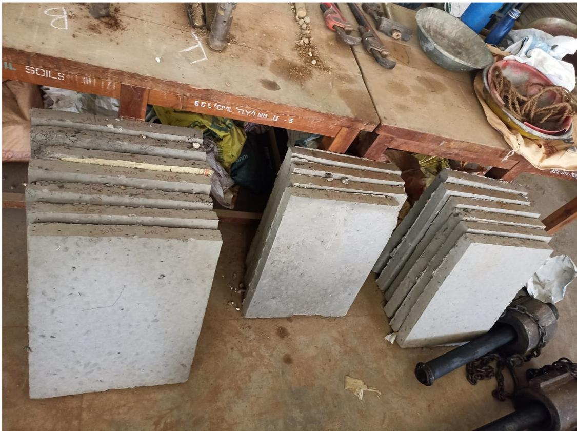
Figure 4: Ambient curing of geopolymer concrete slabs.
