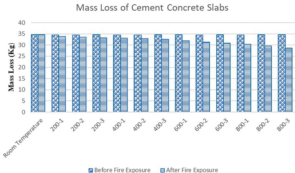
Figure 12: Mass loss of cement concrete slabs subjected to different temperature and duration.
