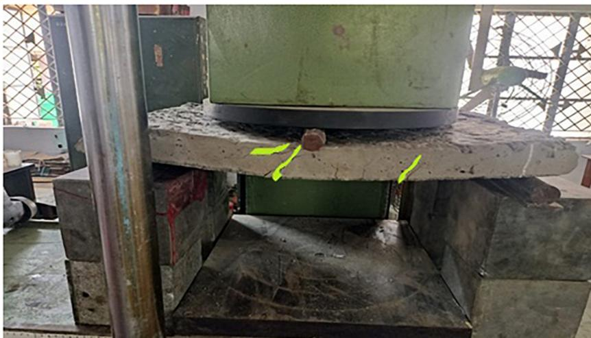
**Figure 17:** Failure mode of fire damaged CC slabs wrapping with BFRP laminates.
