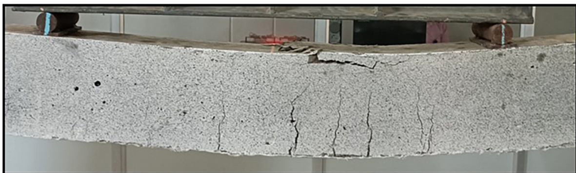
Figure 19: Failure pattern of ECC layered beam with fiber mesh.
