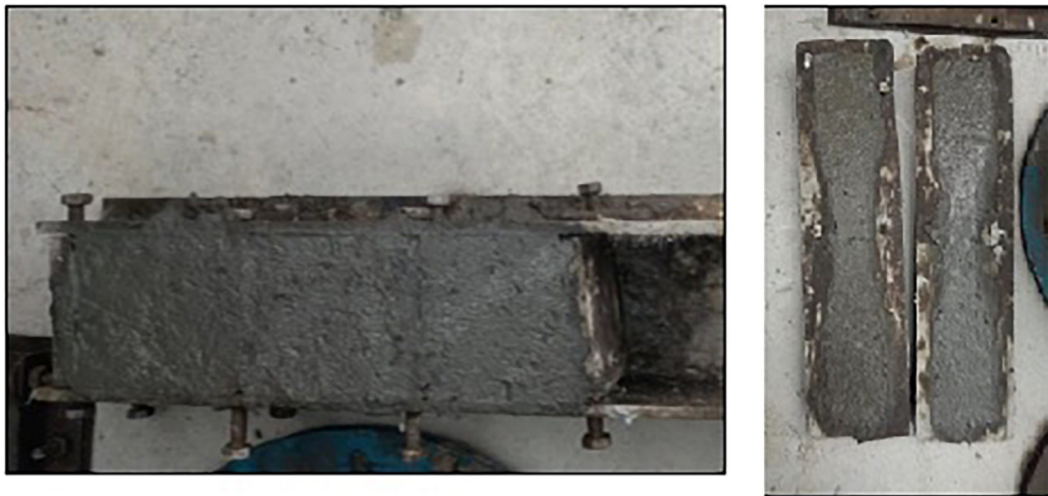
Figure 4: Preparation of mortar cubes and dog-bone specimen.
