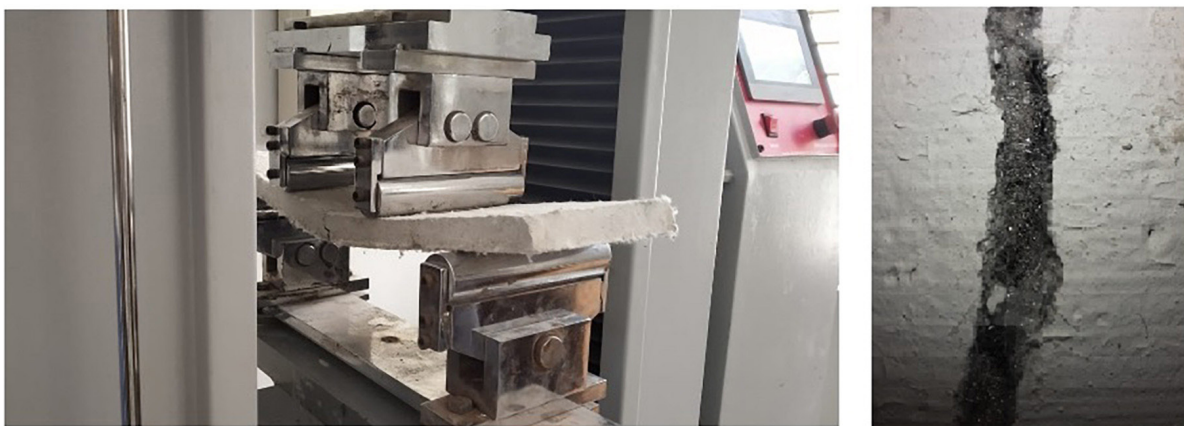
Figure 17: Failure pattern of laminate specimen.
