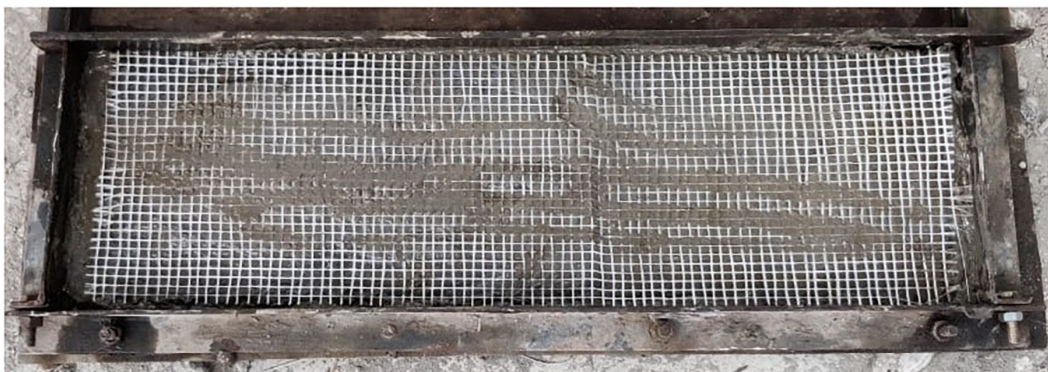
Figure 5: AR glass fiber mesh placed in laminate plate.
