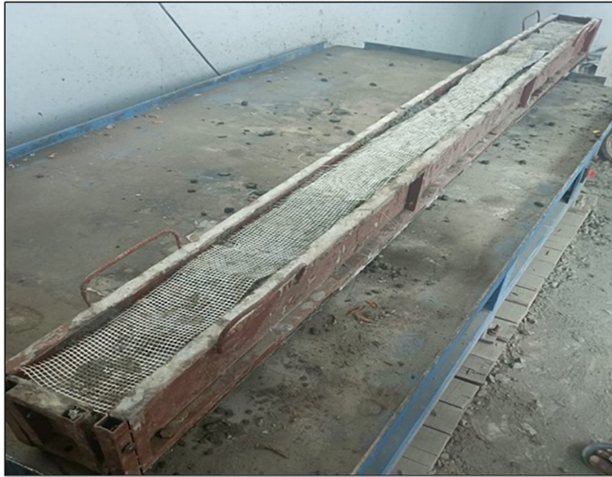
Figure 6: AR glass fiber mesh placed in ECC layered beam.
