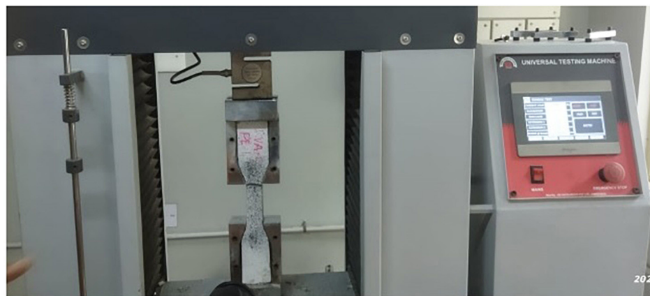
Figure 9: Dog bone specimen dimensions and direct tensile testing machine setup.
